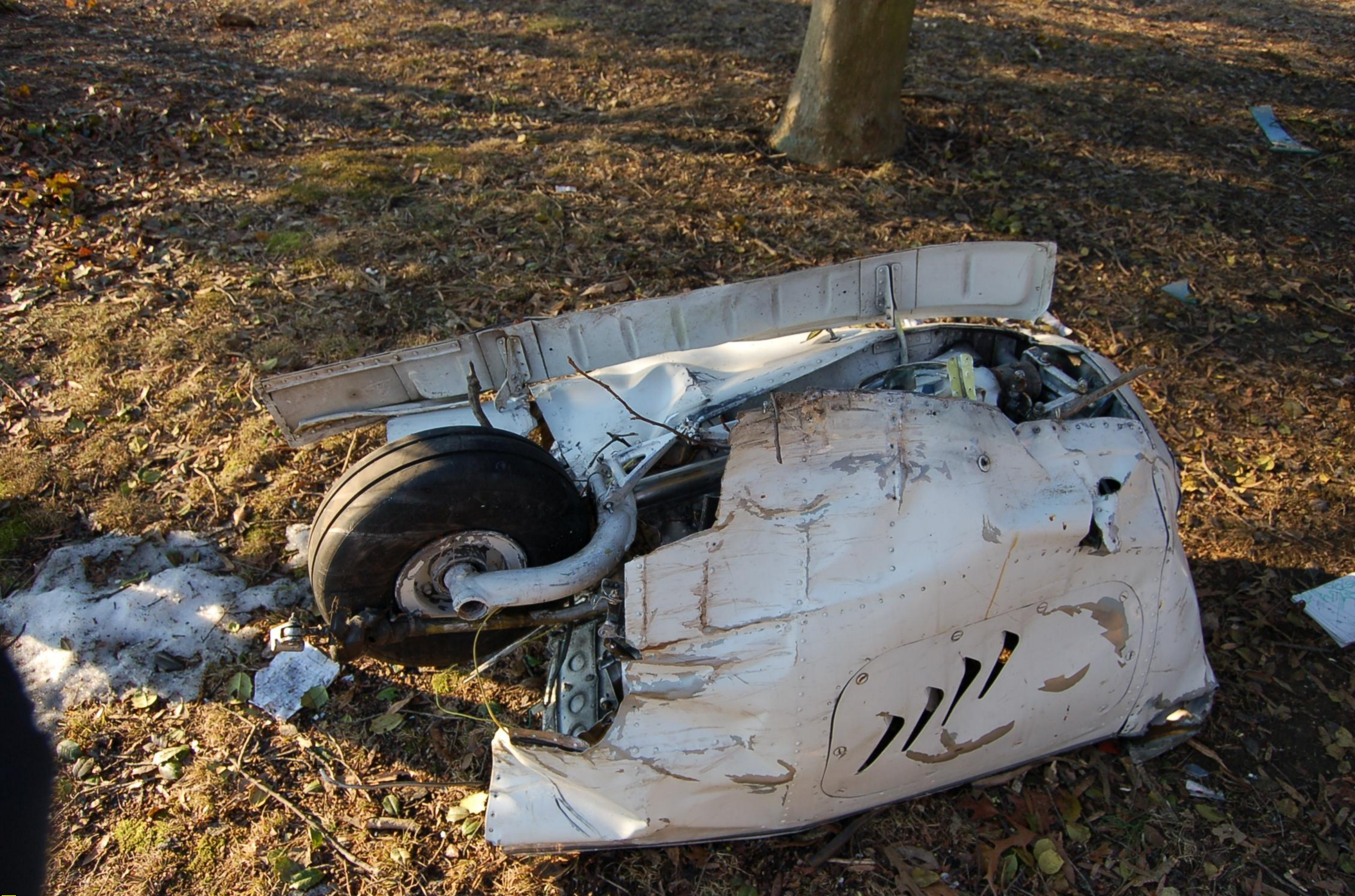
Photograph # 5 – Close-up view of separated nose section with gear assembly.
