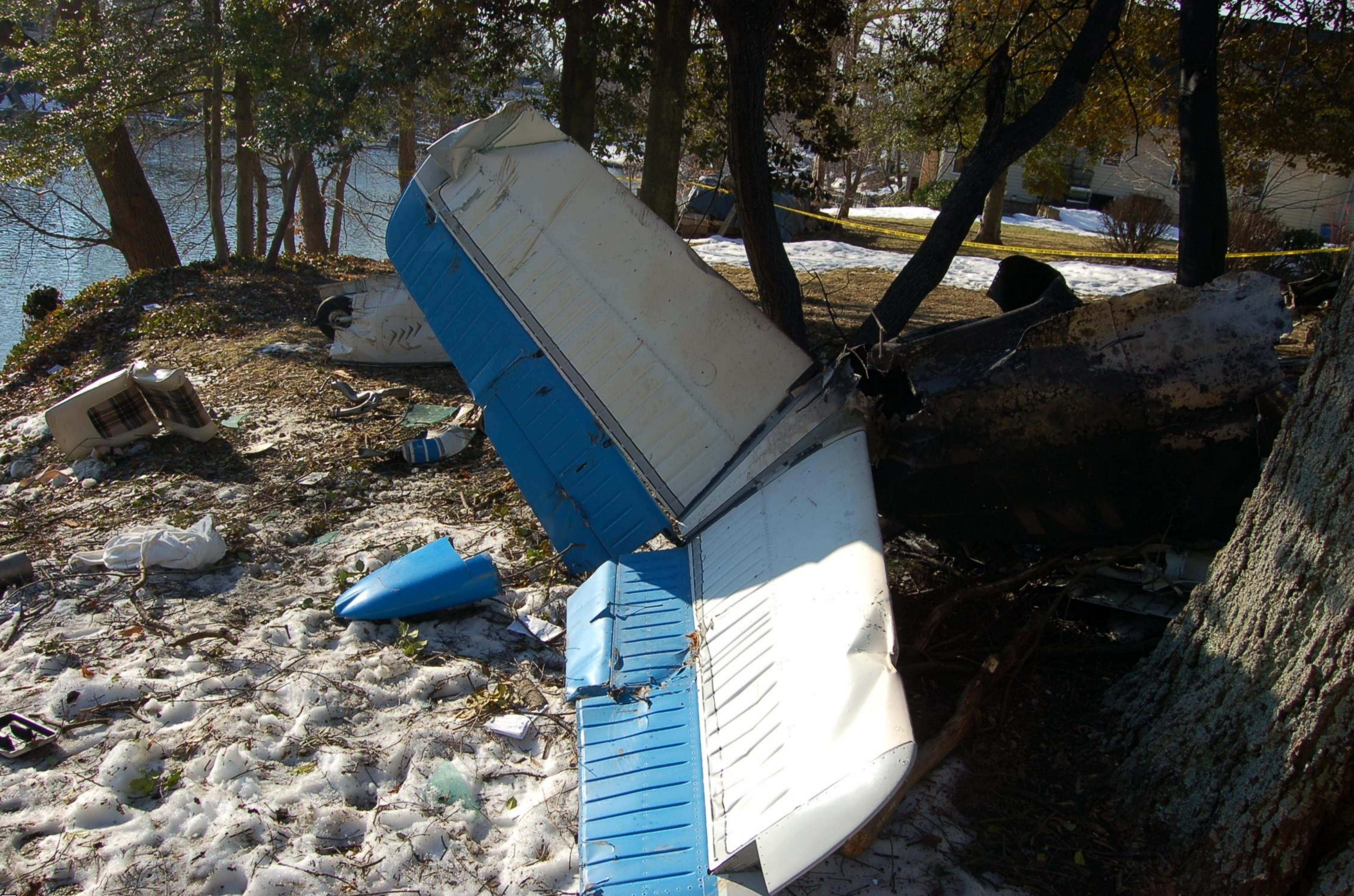
Photograph # 4 – View of a empennage, with separated pilot seat and separated portion of the nose gear assembly also visible.
