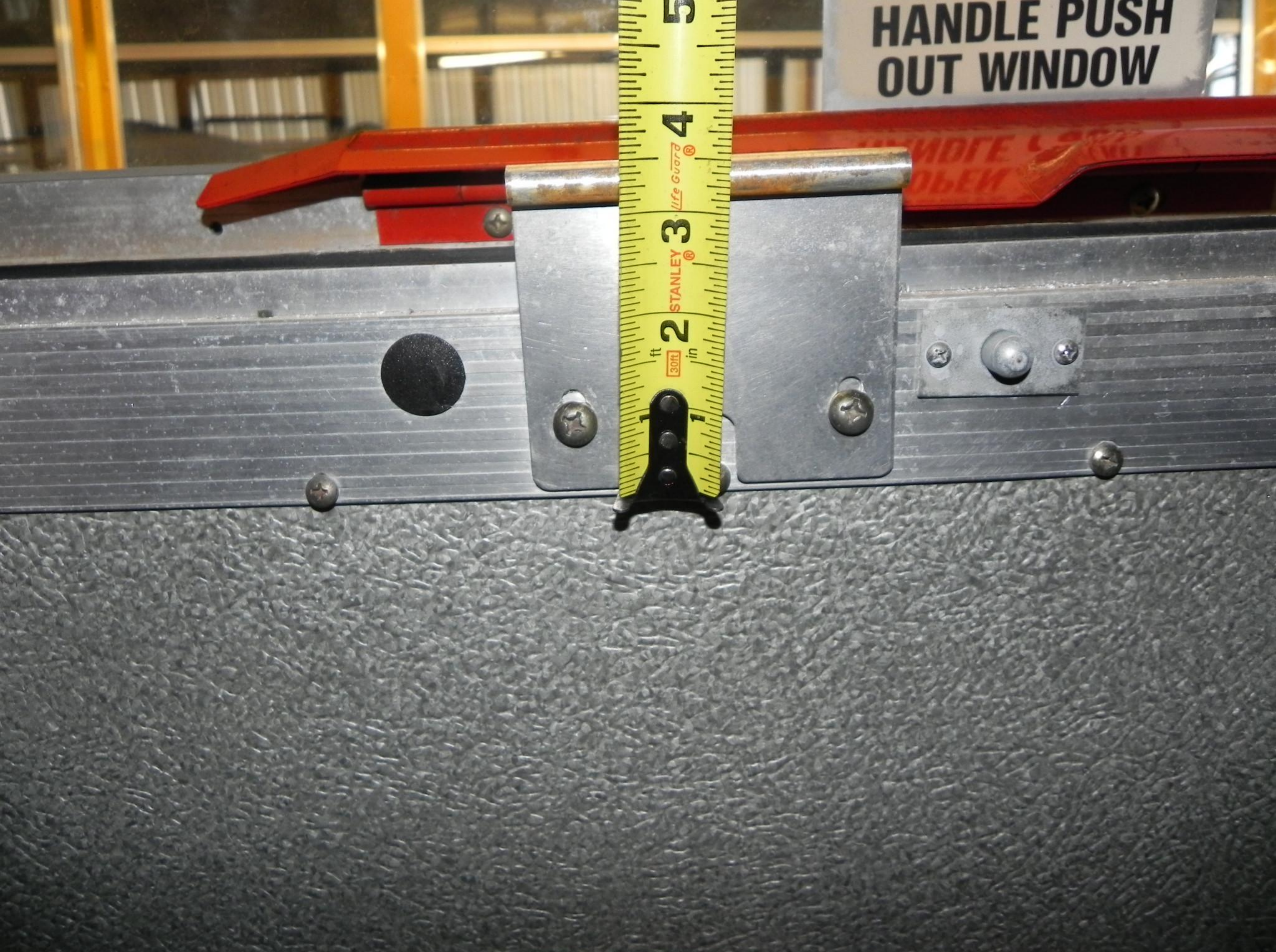
Survival Factors Group Photo 26. View of undamaged rear emergency exit window on 2002 Bluebird 71-passenger school bus showing height of raised latch tab at base of window.
