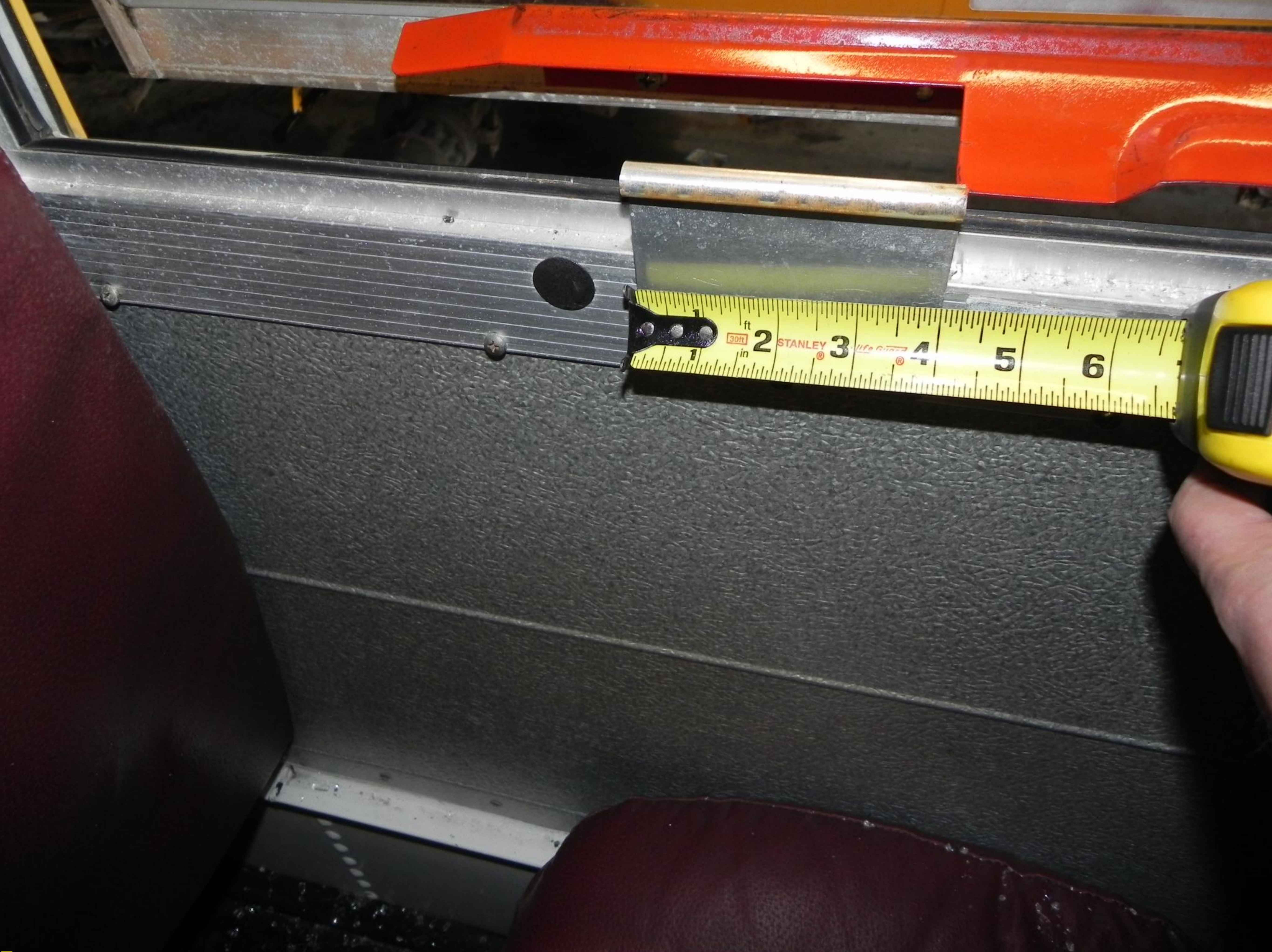
Survival Factors Group Photo 25. View of undamaged rear emergency exit window on 2003 Bluebird 71-passenger school bus showing width of raised latch tab at base of window.
