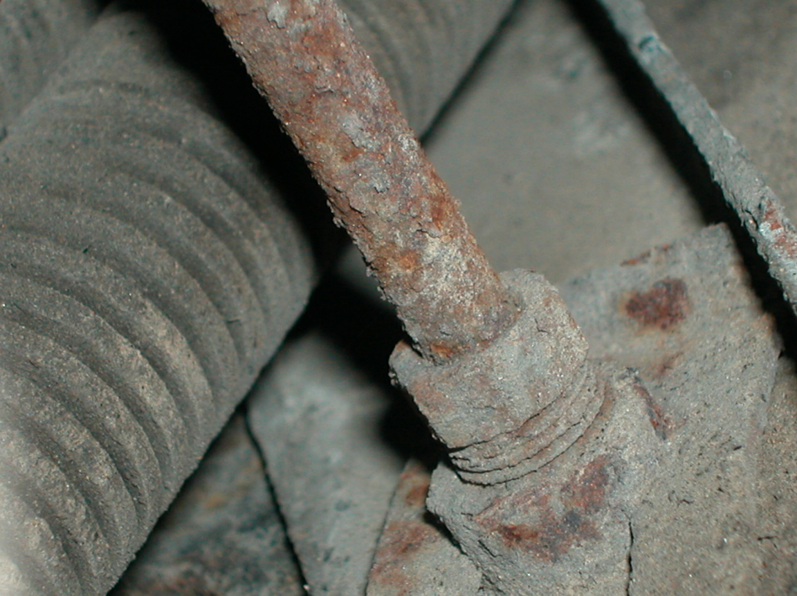
Vehicle Photo 16 – 2001 Blue Bird School Bus, Hydraulic Brake Line for Left Front Wheel
