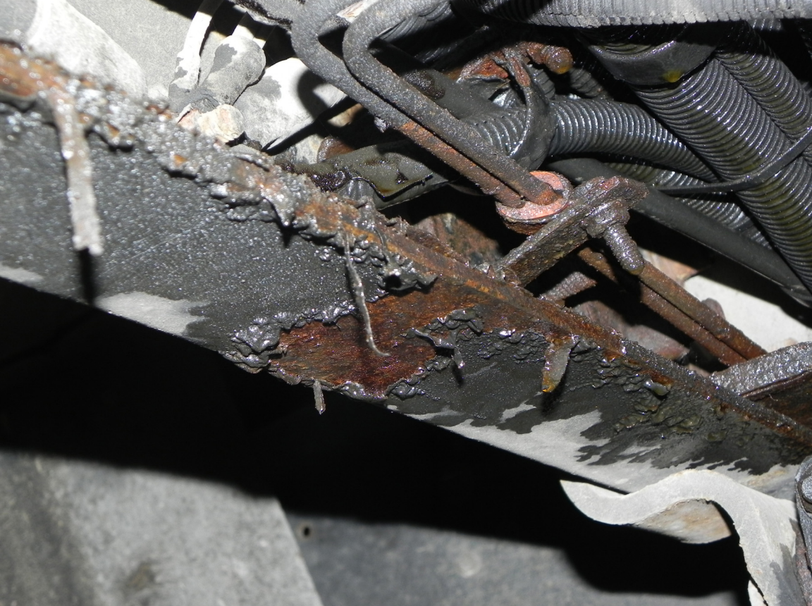
Vehicle Photo 11 – 2003 Blue Bird School Bus, Leaking Hydraulic Brake Lines, View 2
