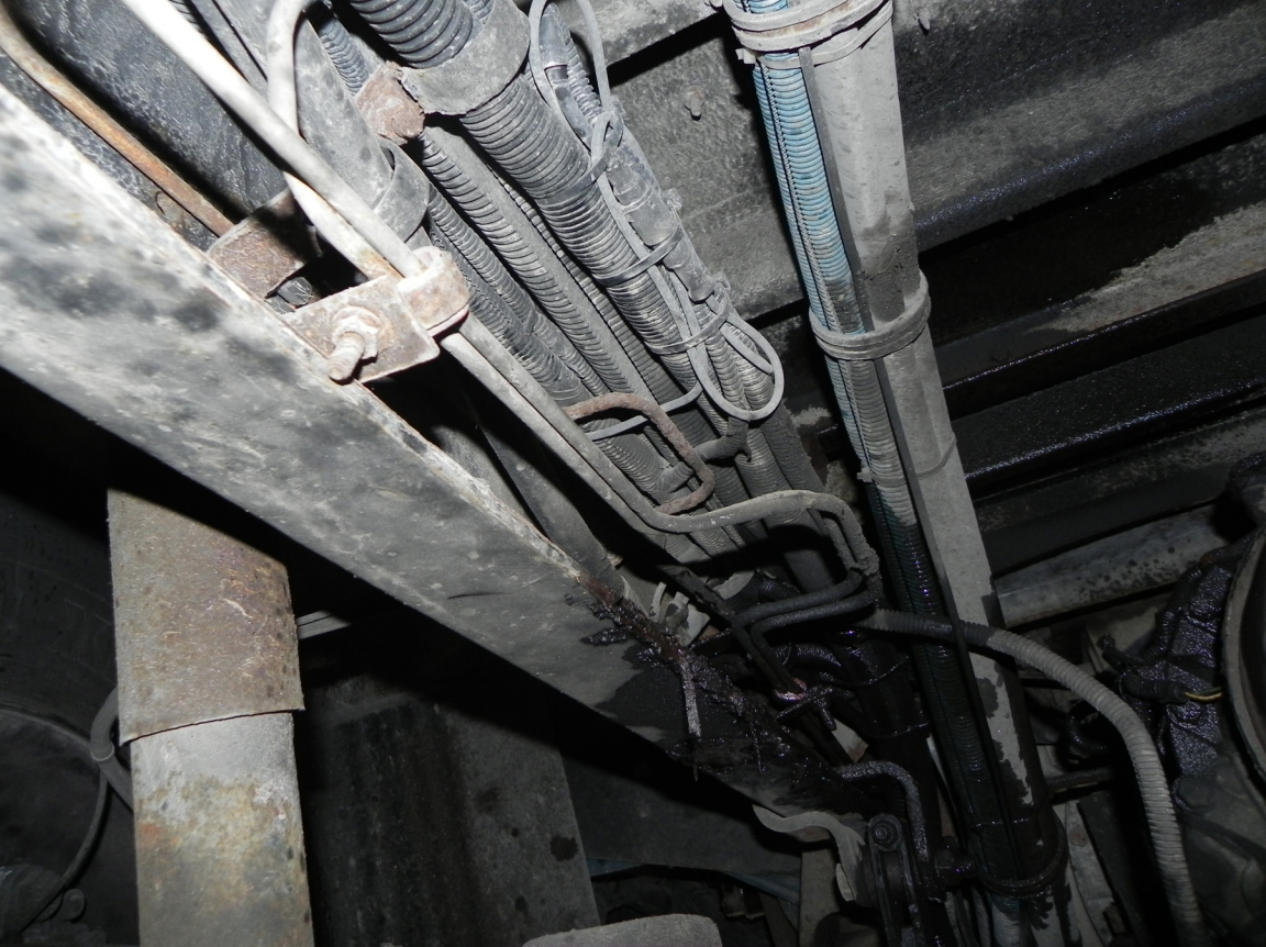
Vehicle Photo 10 – 2003 Blue Bird School Bus, Leaking Hydraulic Brake Lines, View 1
