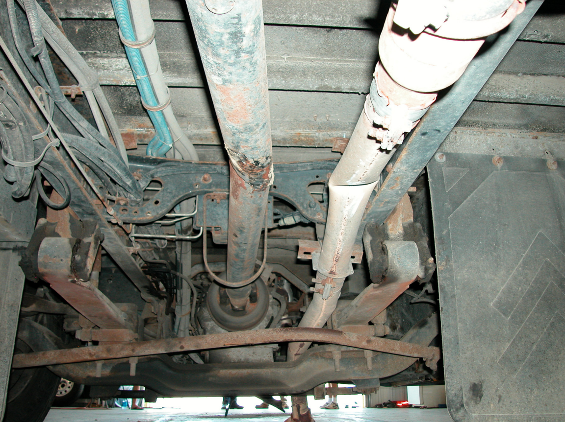
Vehicle Photo 7 – 2003 Blue Bird School Bus, Center Undercarriage Damage
