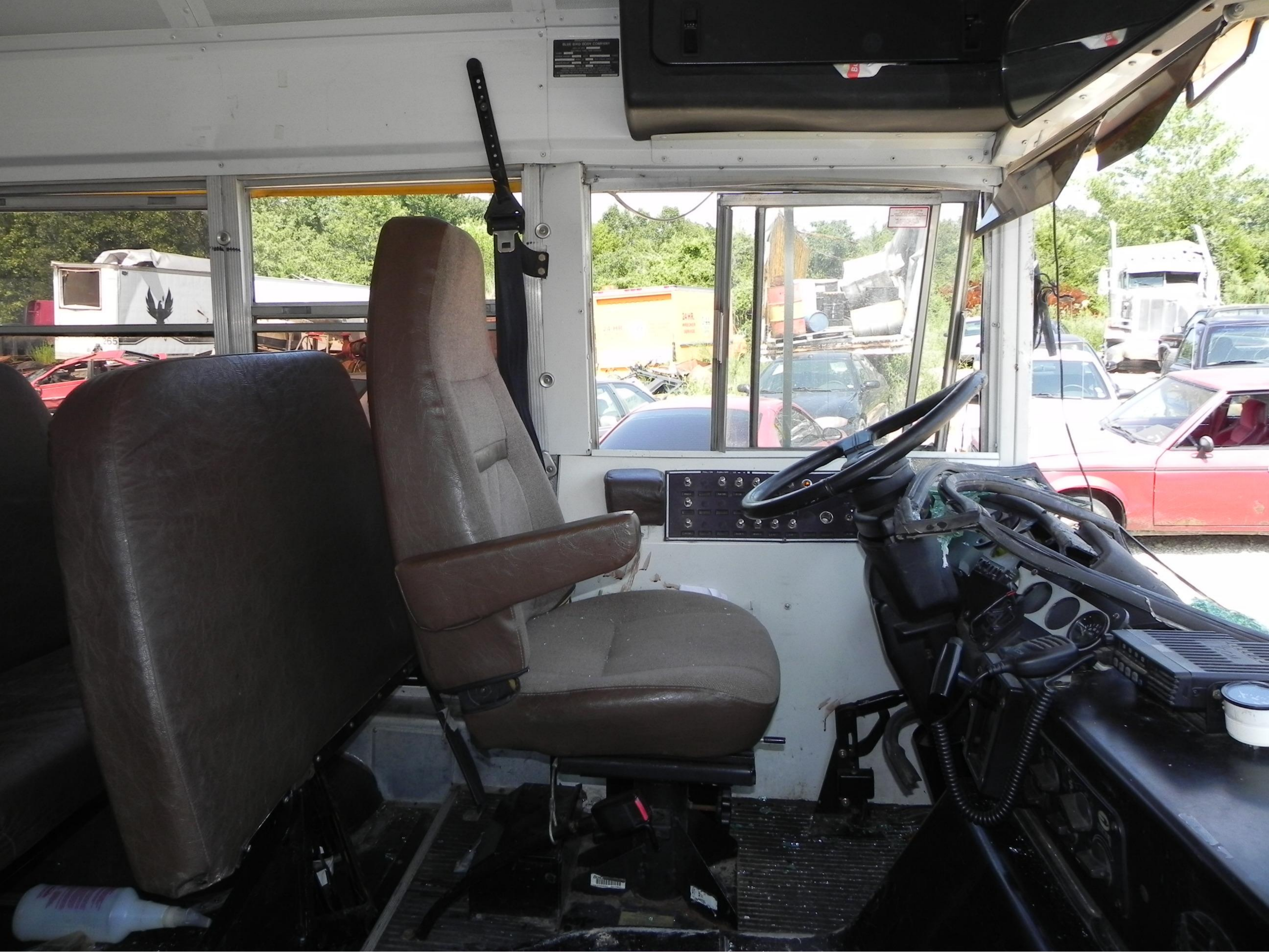
Survival Factors Group. Photo 22. Interior view of driver seating area of 2001 Bluebird school bus showing deformed steering wheel. (NTSB Photograph taken on 08/08/10)
