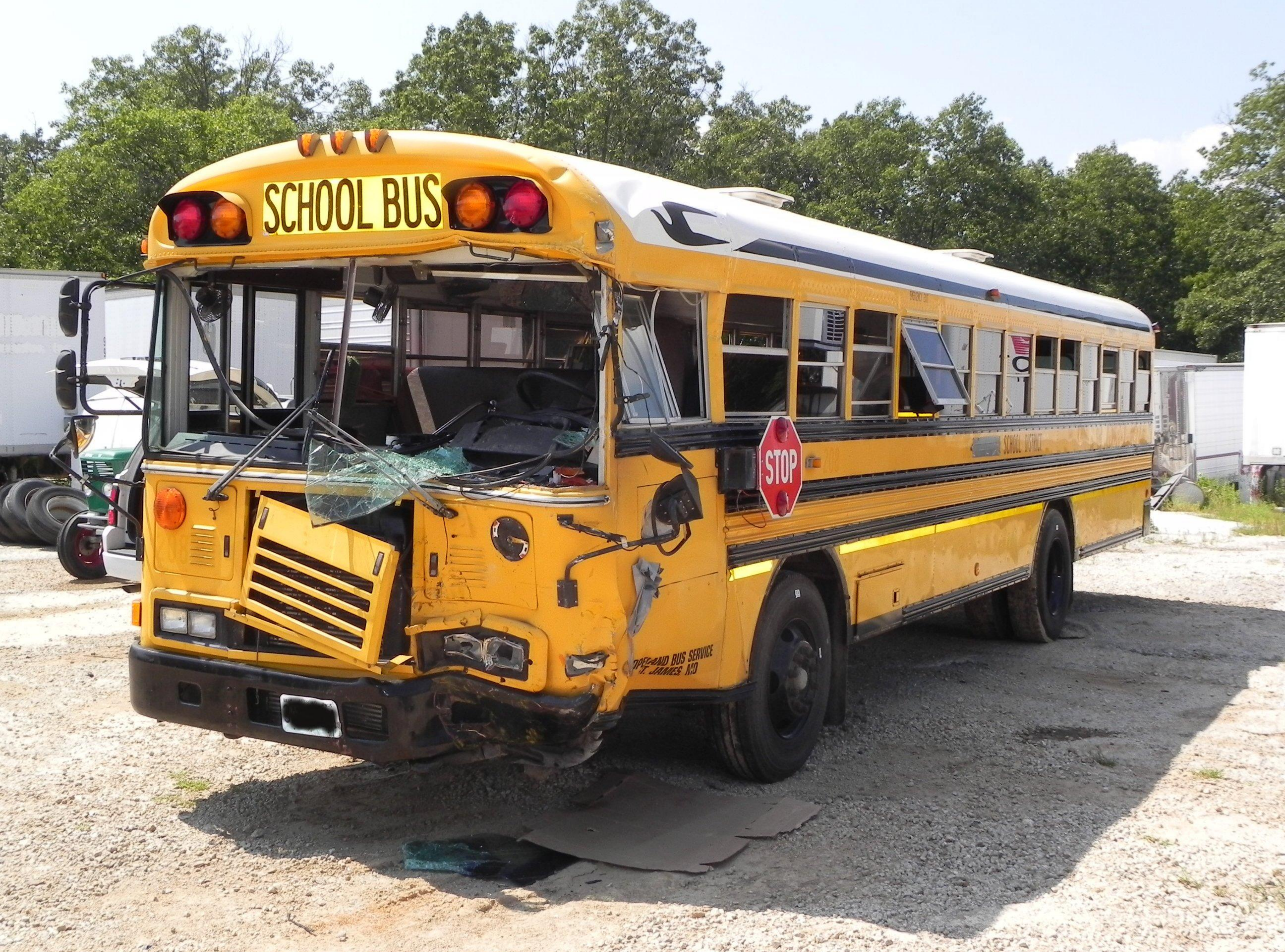
Survival Factors Group. Photo 21. Front left angle view of deformation to 2001 Bluebird school bus from striking 2003 Bluebird school bus. (NTSB Photograph taken on 08/08/10)
