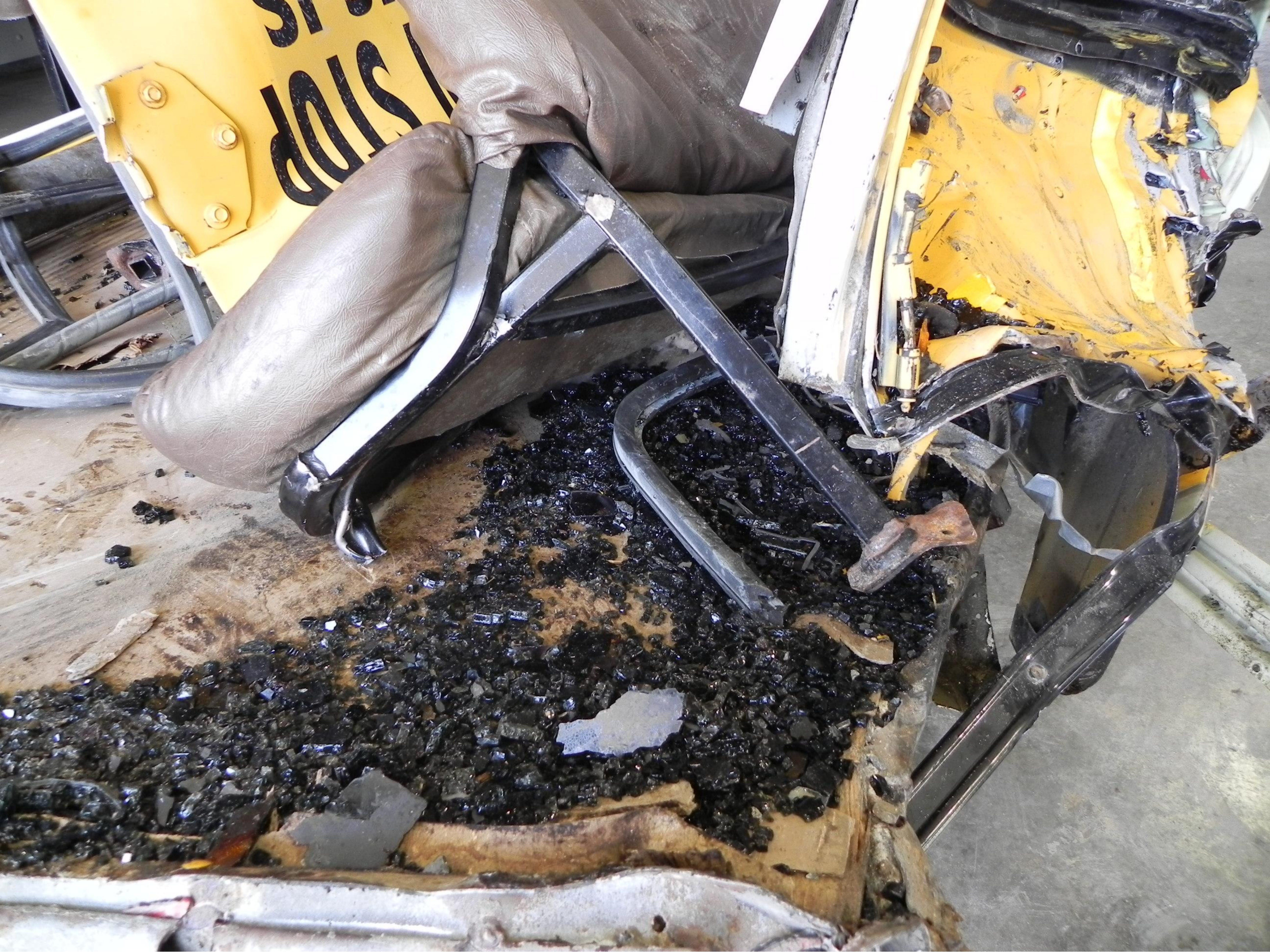
Survival Factors Group. Photo 19. Close-up view of cut and bent rear seat floor anchors of 2003 Bluebird school bus. (NTSB Photograph taken on 08/08/10)
