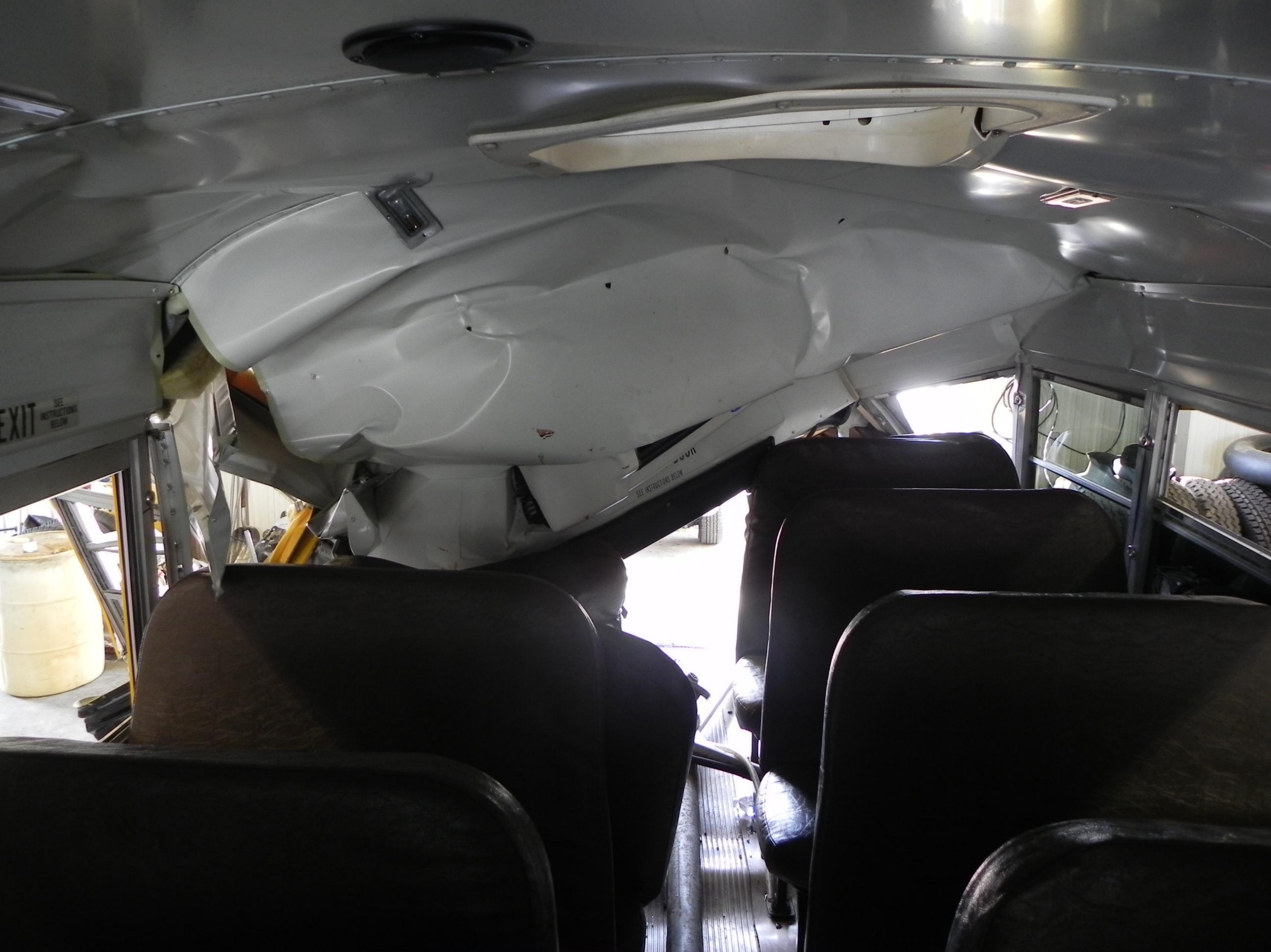
Survival Factors Group. Photo 16. Closer-up view from front to rear of 2003 Bluebird school bus showing intrusion to rear and roof. (NTSB Photograph taken on 08/08/10)
