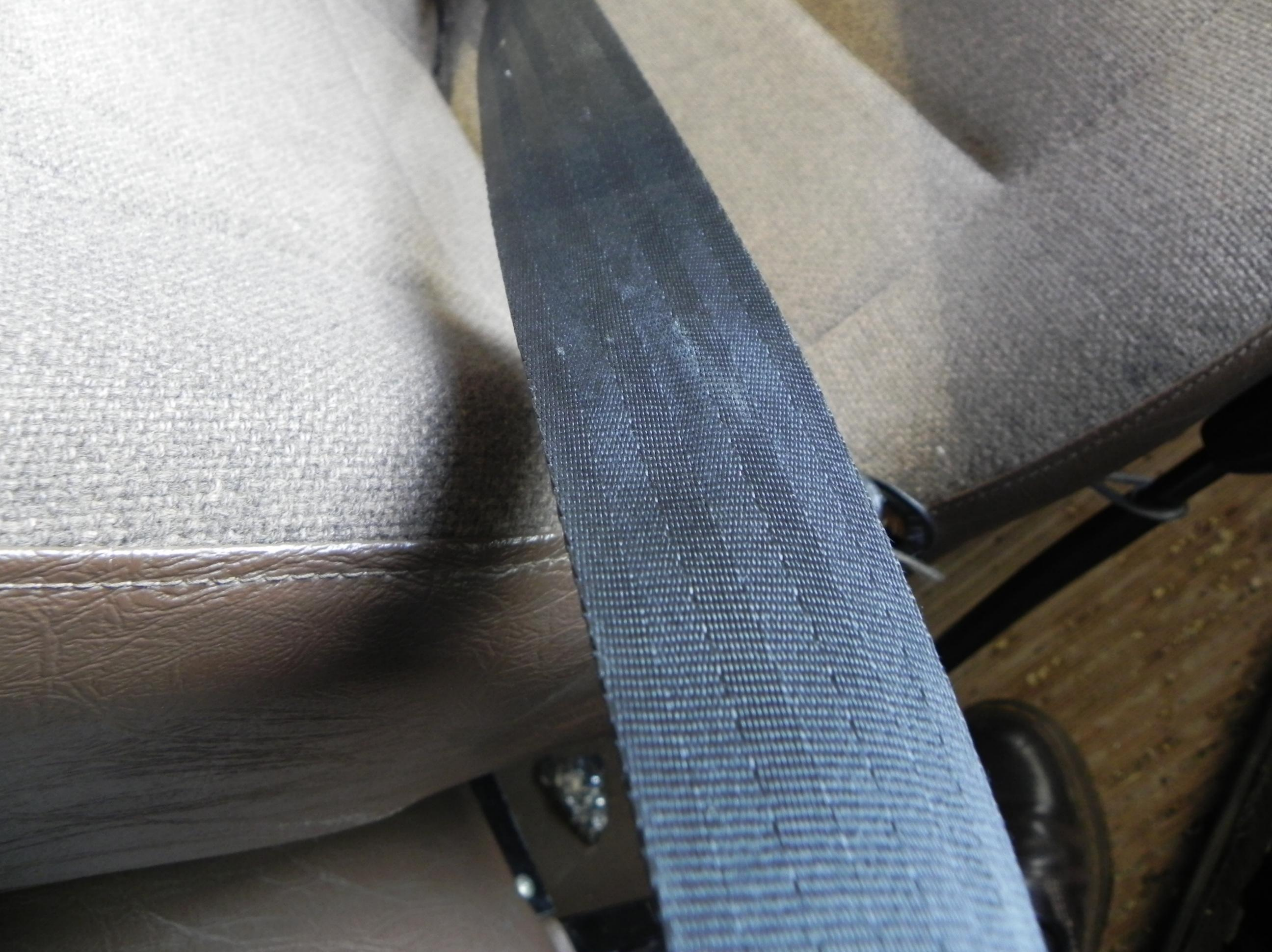
Survival Factors Group. Photo 15. Close-up of heat abrasion to 2003 Bluebird school bus driver's seatbelt. (NTSB Photograph taken on 08/08/10)
