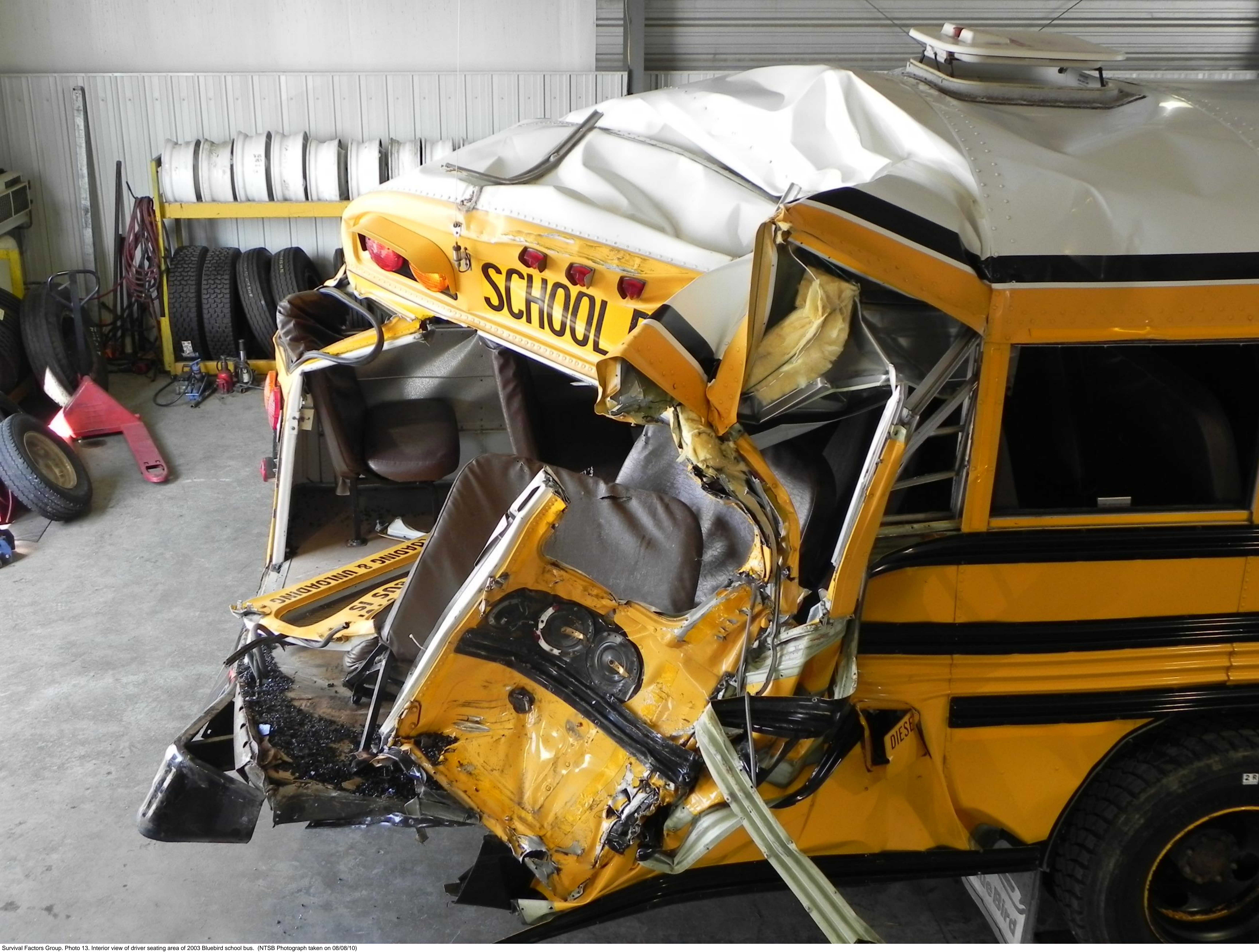
Survival Factors Group. Photo 13. Interior view of driver seating area of 2003 Bluebird school bus. (NTSB Photograph taken on 08/08/10)
