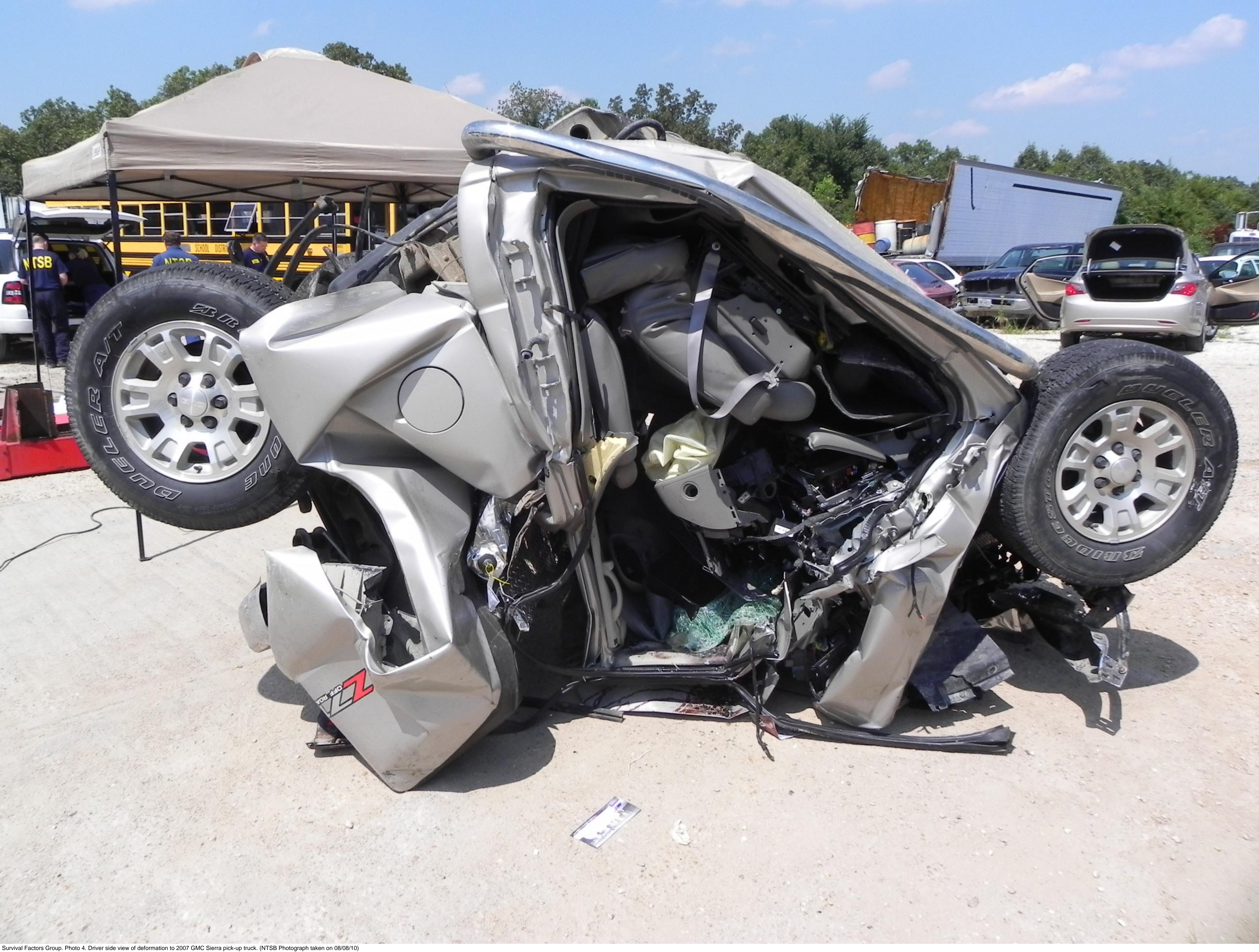
Survival Factors Group. Photo 4. Driver side view of deformation to 2007 GMC Sierra pick-up truck. (NTSB Photograph taken on 08/08/10)
