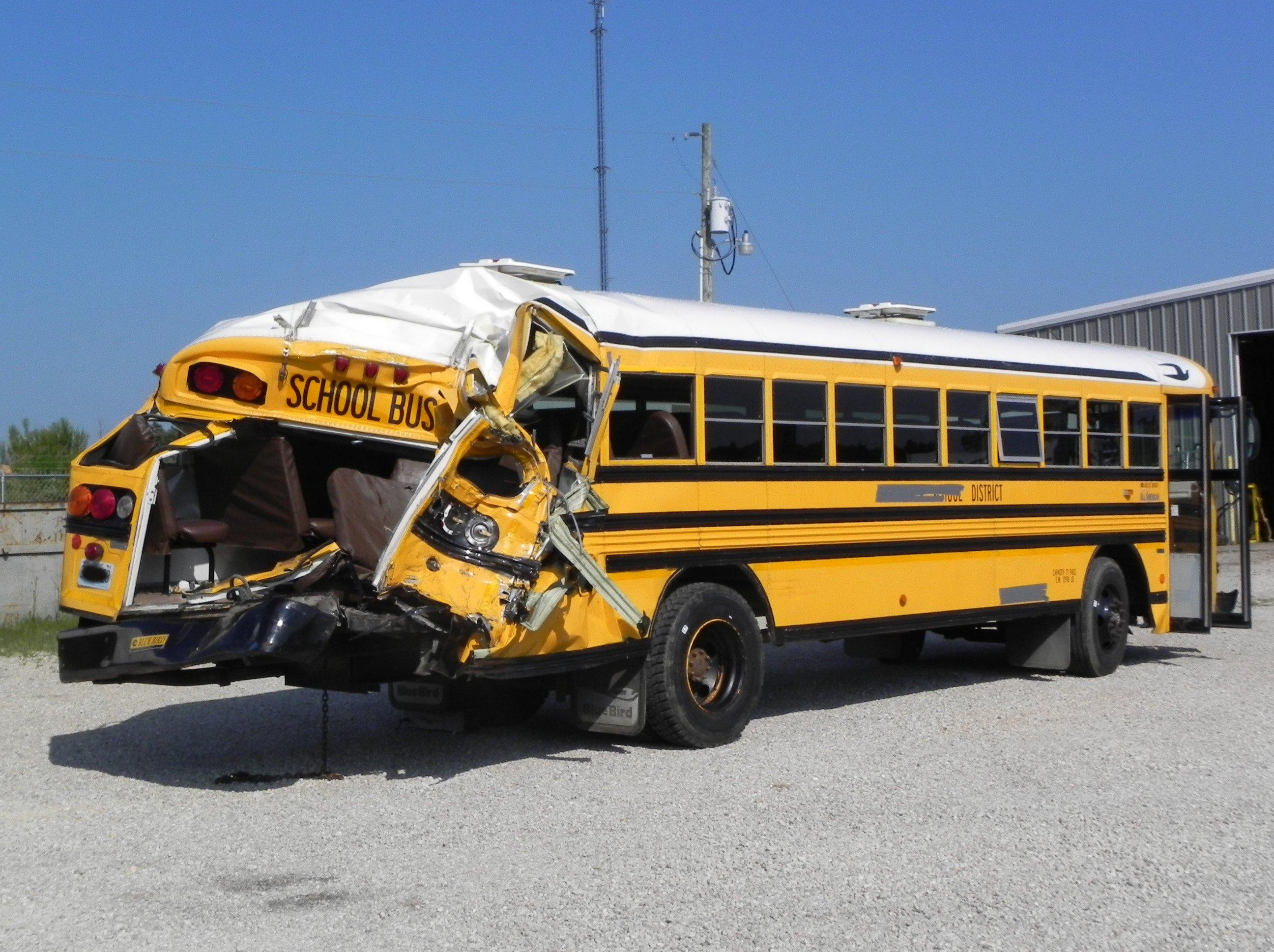
Survival Factors Group. Photo 12. Rear right angle view of deformation to rear of 2003 Bluebird school bus. (NTSB Photograph taken on 08/08/10)
