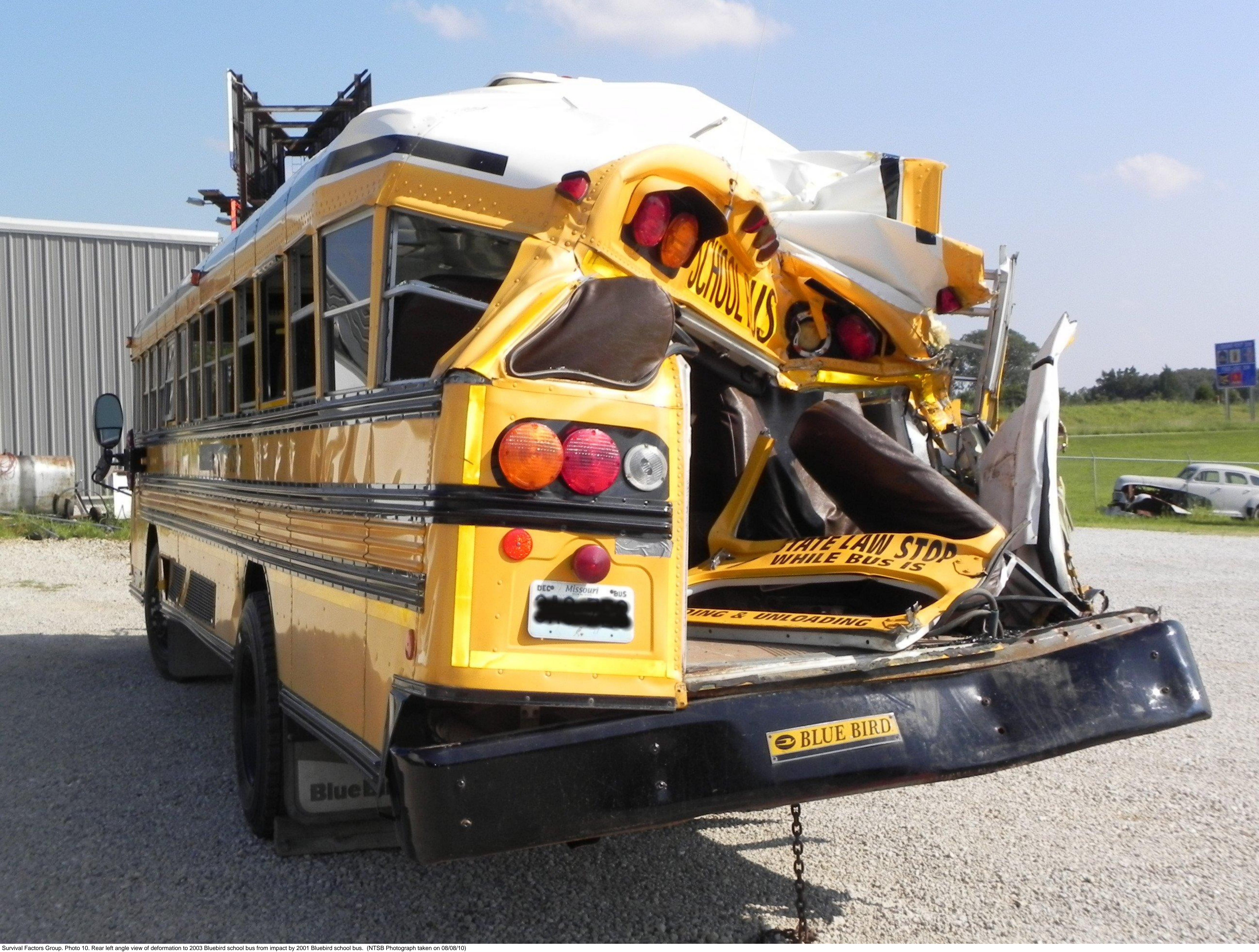
Survival Factors Group. Photo 10. Rear left angle view of deformation to 2003 Bluebird school bus from impact by 2001 Bluebird school bus. (NTSB Photograph taken on 08/08/10)
