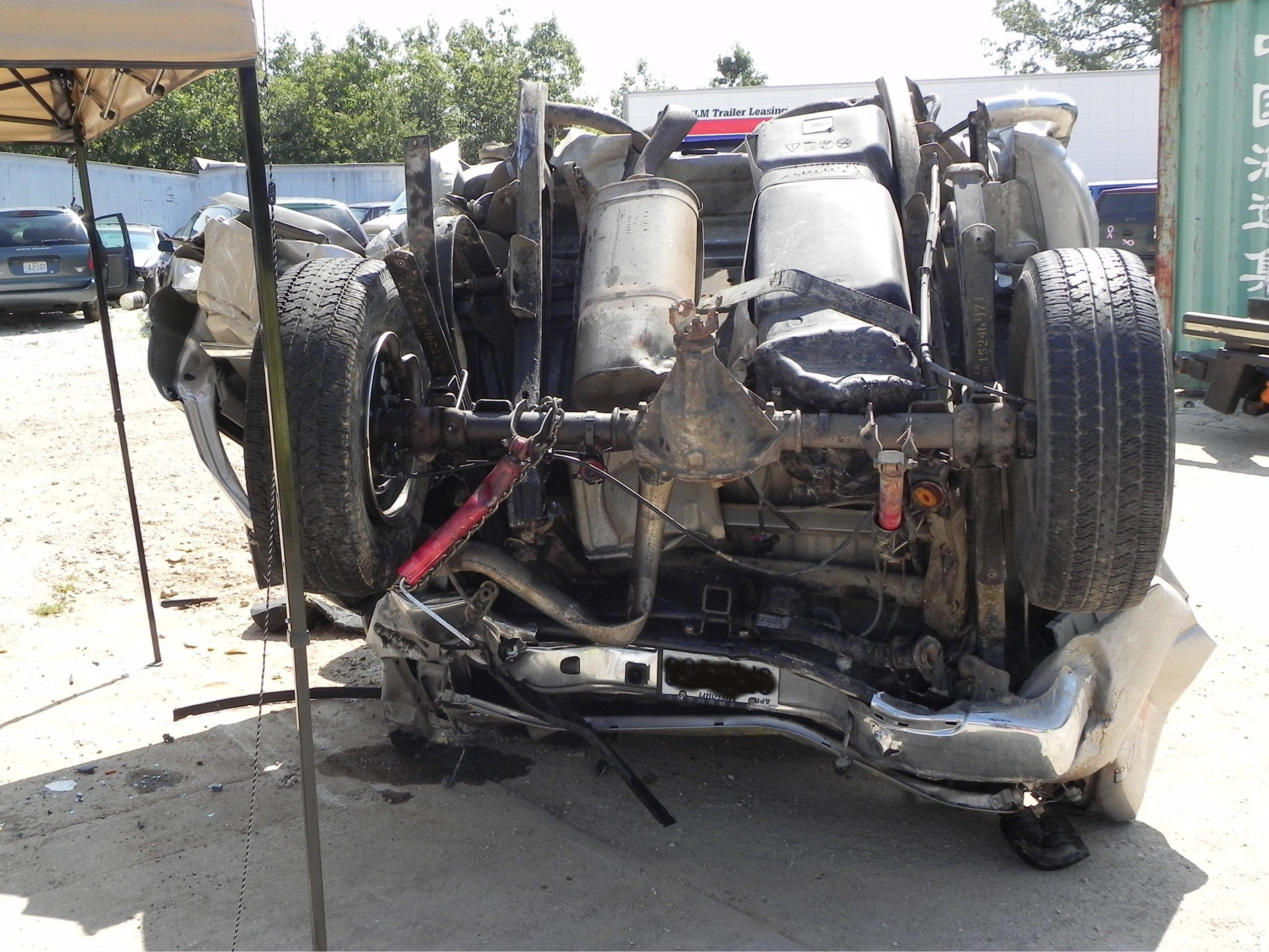
Survival Factors Group. Photo 7. Front right angle view of deformation to 2007 GMC Sierra. (NTSB Photograph taken on 08/08/10)
