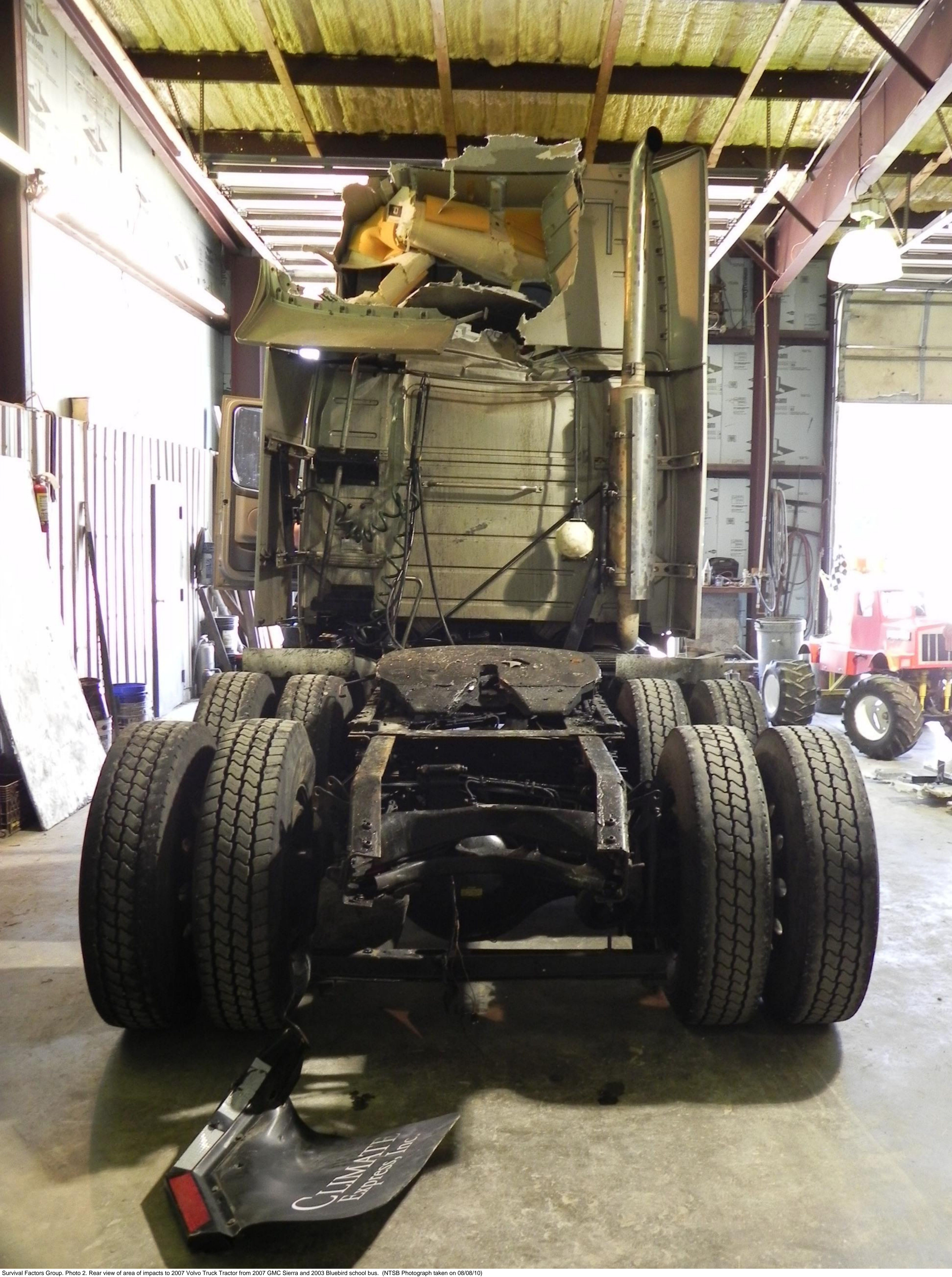
Survival Factors Group. Photo 2. Rear view of area of impacts to 2007 Volvo Truck Tractor from 2007 GMC Sierra and 2003 Bluebird school bus. (NTSB Photograph taken on 08/08/10)
