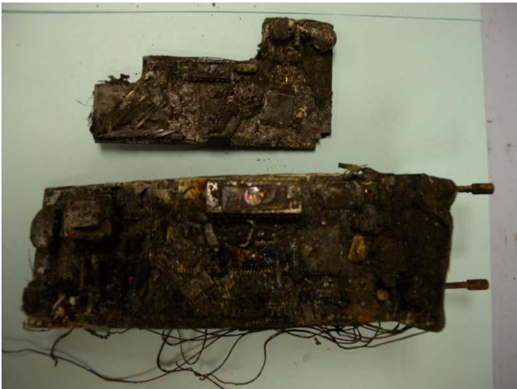
Figure 2 - Close-up of EDM circuit cards
