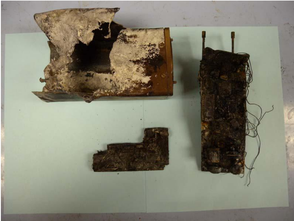
Figure 1 - EDM circuit cards with external case removed
