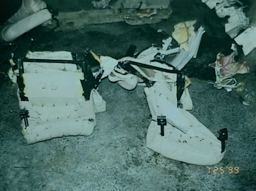
Airworthiness - Photo 16. View of the seat back structure of the aft-facing passenger seats in row 2. Note that the structure is bulged outward (forward relative to their normal installation in airplane). (NTSB-A2)
