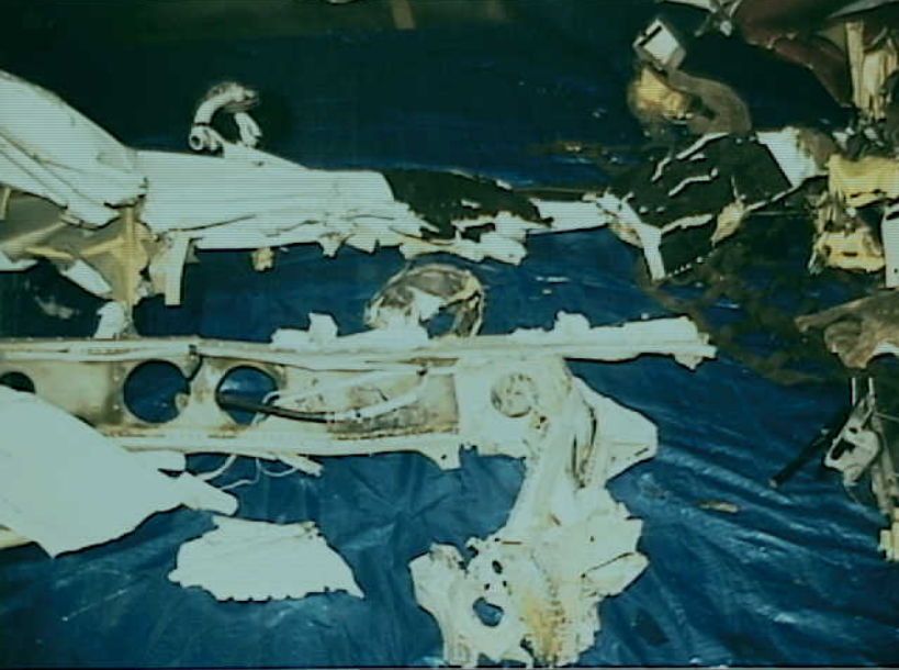
Airworthiness - Photo 7. Close-up view of the right wing spar area near 90-degree forward bend. Right main landing gear trunion (shown in foreground) is normally installed in this area. Note damage to the spar web in this area. (NTSB-I22)
