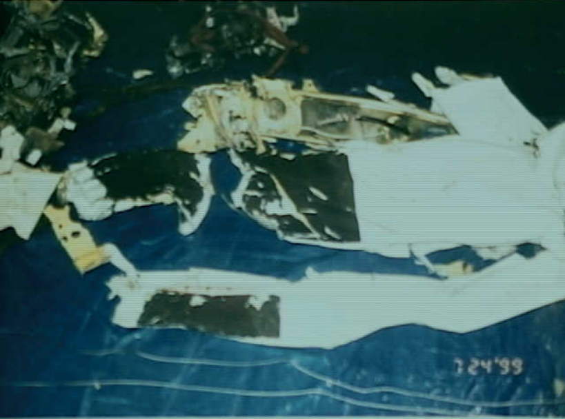
Airworthiness - Photo 6. View off the inboard section of the right wing (view from forward looking aft). Note damage to main spar and the 90-degree forward bend (foreground) (NTSB-C14)
