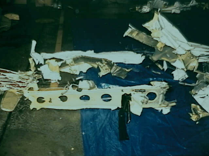
Airworthiness - Photo 5. View of the inboard section of the right wing (view from aft looking forward). Note damage to main spar (background). Also note entire left flap (foreground) and lack of bulging or bowing
