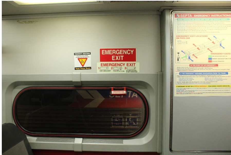
Figure 9 Photograph of the emergency exit window markings as seen from the interior of the train car. (Source: NTSB)
