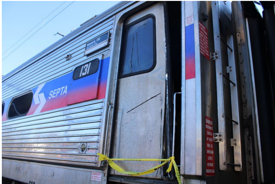
Figure 5 Photograph of the platform door on Car 131 damaged during the fire department's forcible entry into the train car. (Source: NTSB)
