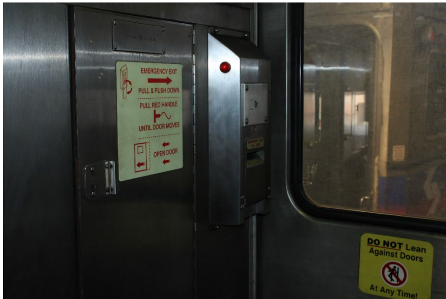
Figure 7 Photograph of the emergency instructions and the emergency door release inside one of the train cars. (Source: NTSB)
