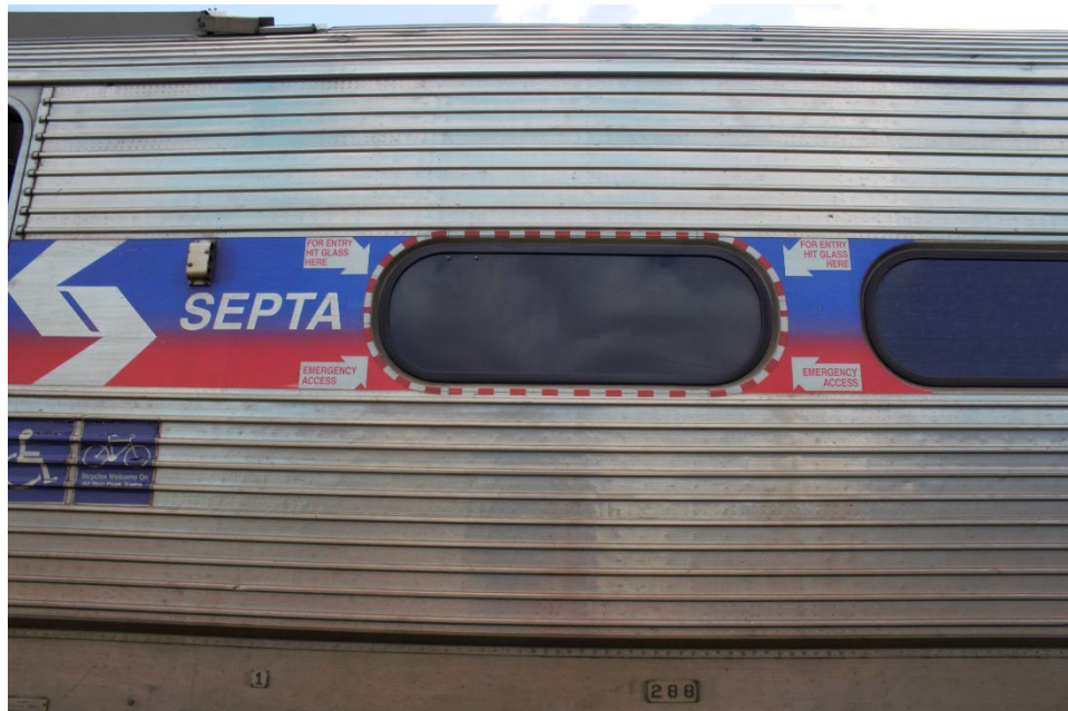
Figure 8 Photograph showing the emergency exit window markings as seen from the exterior of the train. (Source: NTSB)
