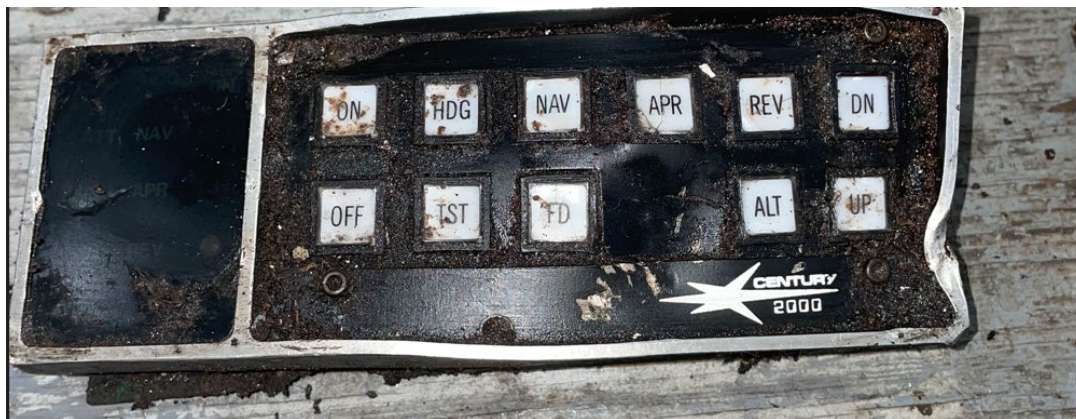
Figure 5: Century 2000 AP control panel after cleaning.
