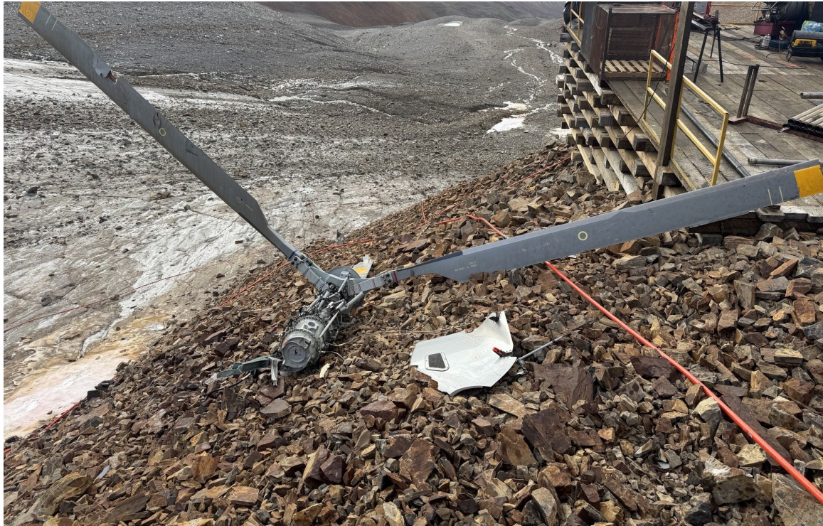
Photograph 2 - View of separated main rotor blades. (Courtesy of operator)
