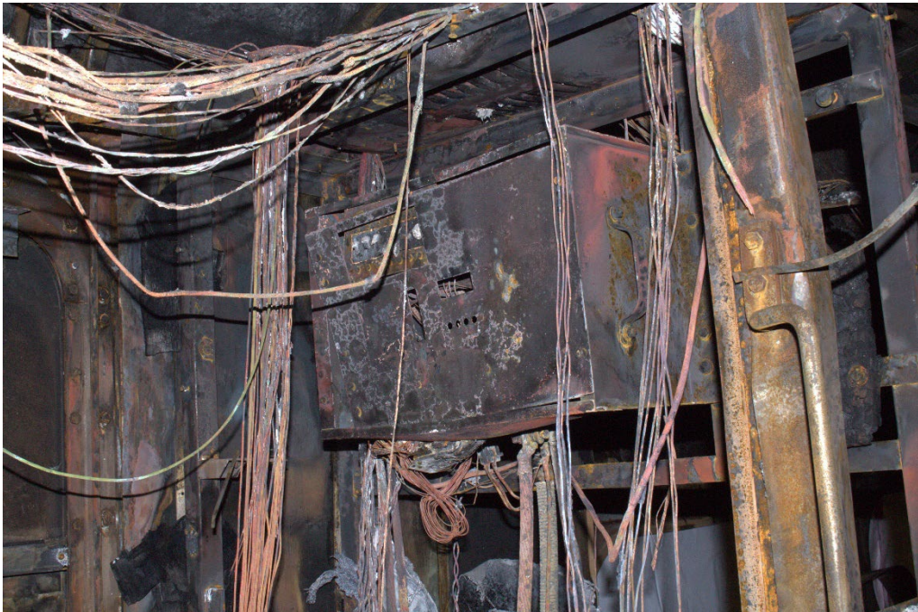
Photo 14 A Closeup of the electronic equipment located within the mid-car partitions after the exterior structure of the partition was burned away. (Source: NTSB)
