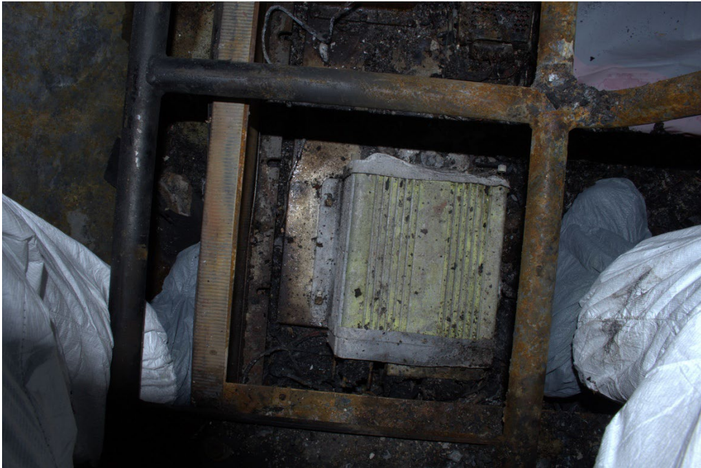
Photo 11 A closeup of the second electronic recorder module, in the position found, that was located underneath what remained of the mid-car seat in Car 132. (Source: NTSB)
