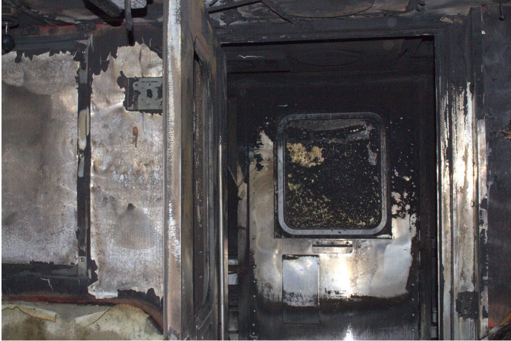
Photo 7 Photograph of the interior end car door in Car 132 and the damage caused by the fire. (Source: NTSB)
