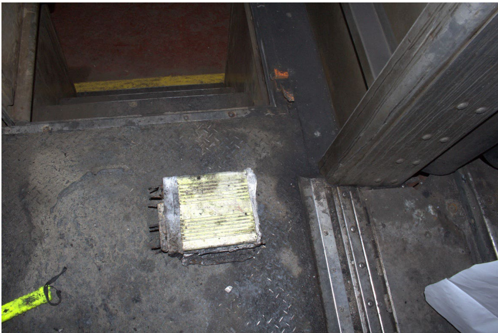
Photo 12 A closeup of the second recorder module after it was removed from underneath the seat by investigators. (Source: NTSB)
