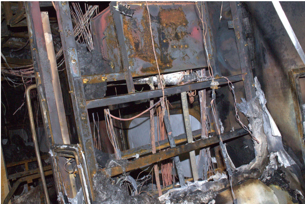
Photo 16 A closeup of the burned partition located the mid-car and adjacent to the seats that was burned completely through the interior of the compartment. (Source: NTSB)
