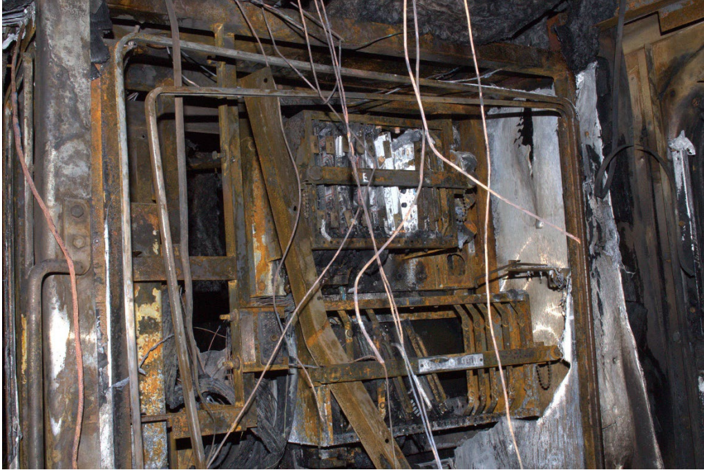
Photo 15 A closeup of the mid-car partition that was burned away during the fire exposing the frame of the interior electronic component compartment. (Source: NTSB)
