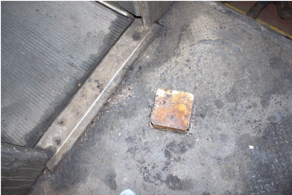
Photo 10 A photograph of the electronic recorder module after it was removed from its location underneath the mid-car seat. (Source: NTSB)
