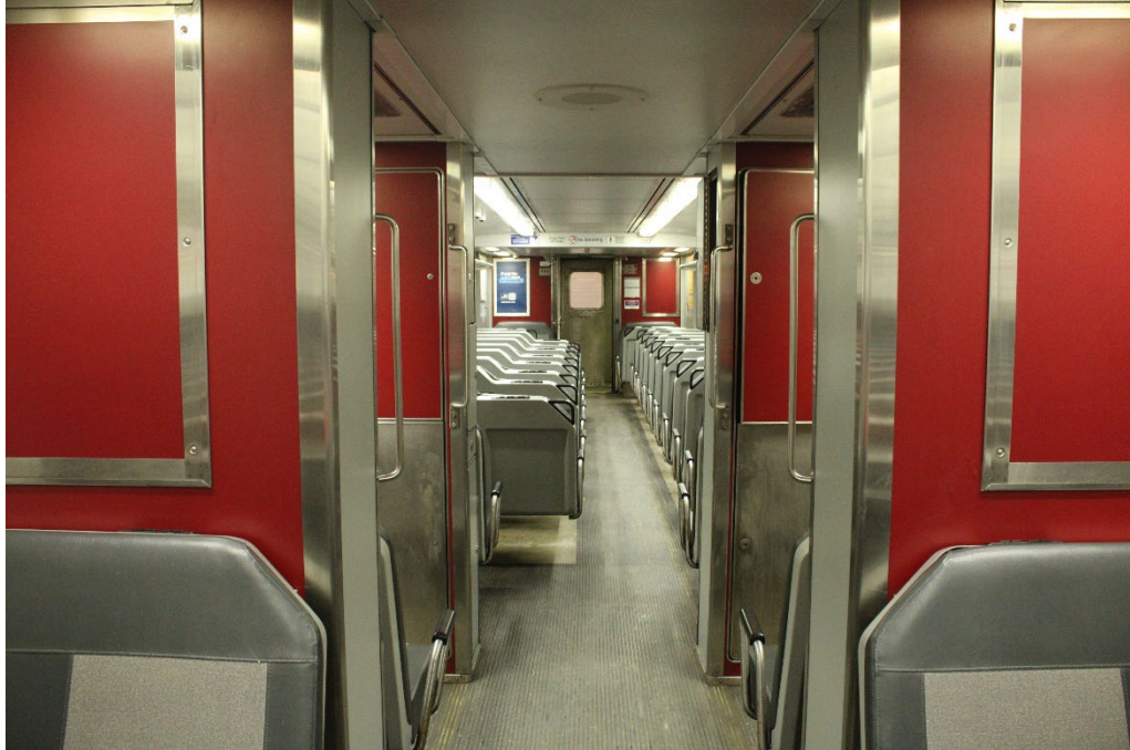
Photo 17 A photograph of the partitions in front and behind the mid-car seats which houses the rail car electronics in the interior space. (Source: NTSB)
