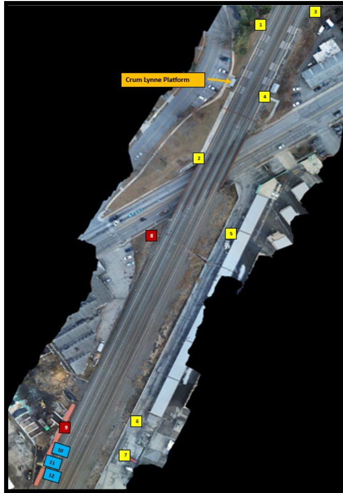
Figure 2 Screen capture of two-dimensional orthomosaic showing the location of the ground control points within the incident scene.
