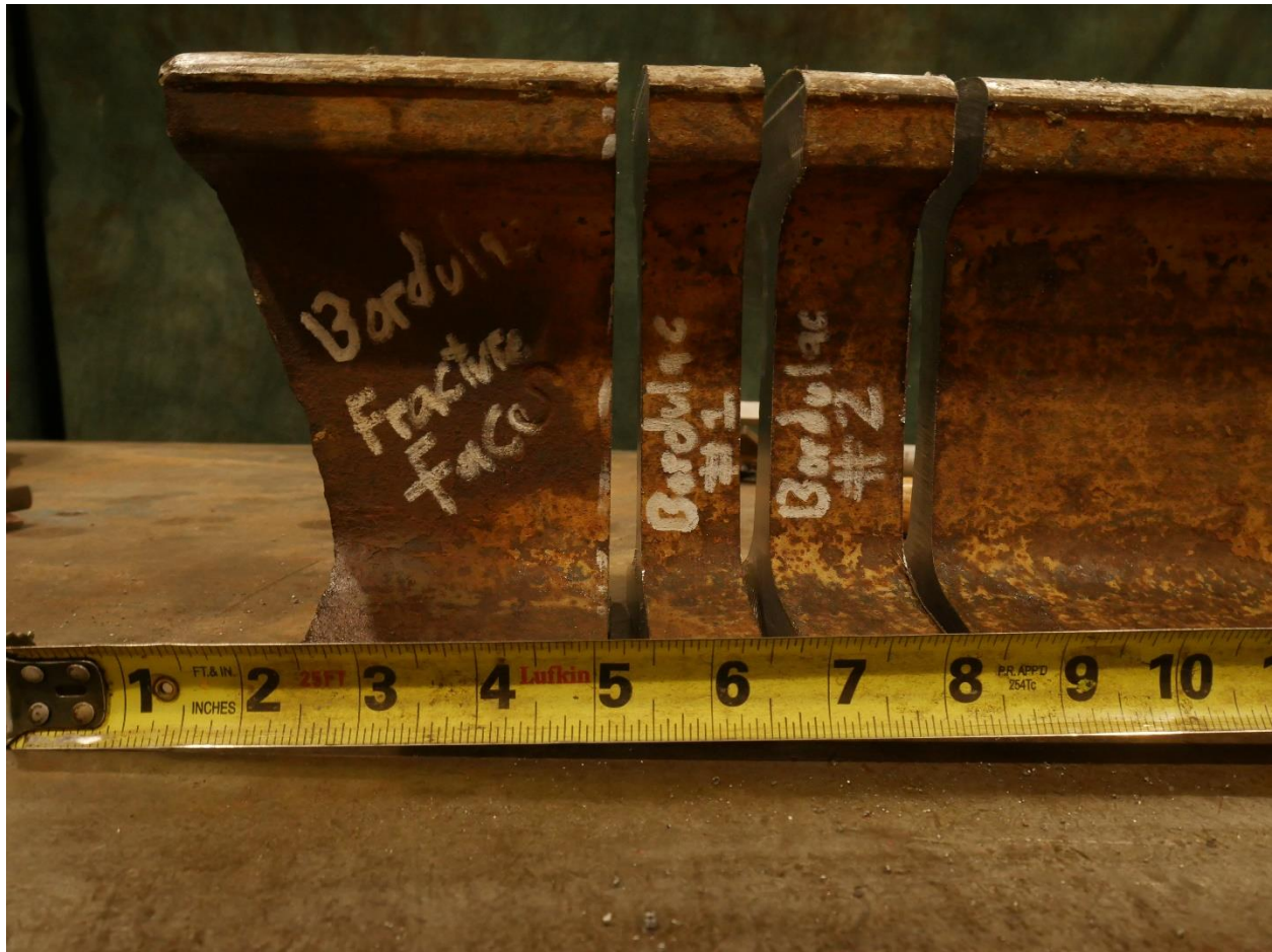
Image 12: The four sections of rail, the fracture face, sample 1, sample 2, and the remainder.
