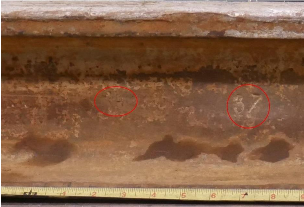
Image 3: Gauge side rail stamp saying “IH” and “37” on opposite side of rail.
