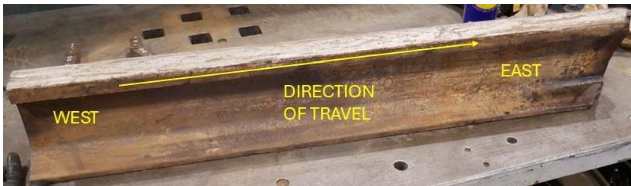
Image 1: The 43" section of rail after being cleaned. The field side is visible.
