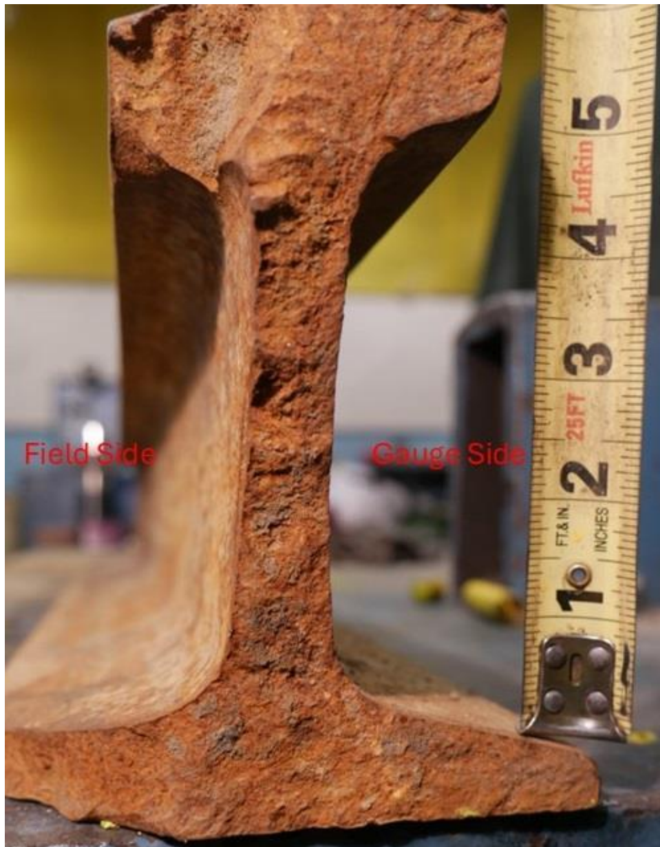
Image 5: The fracture face showing characteristics of brittle fracture, namely a flat surface and chevrons pointing towards the initiation sites.
