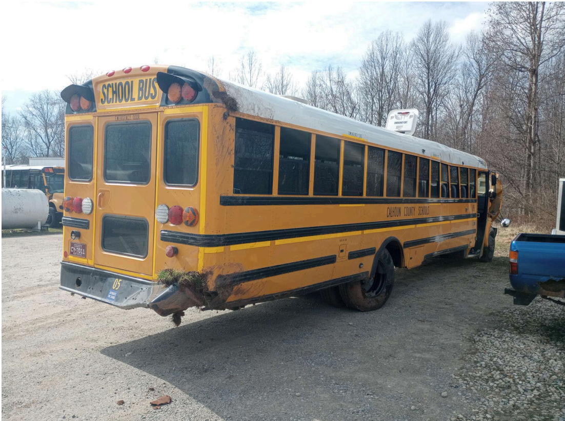
Figure 2 Photo of damage to the rear of bus #5. Source: (West Virginia State Police)
