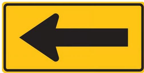
Figure 5. One-direction large arrow sign (W1-6).
