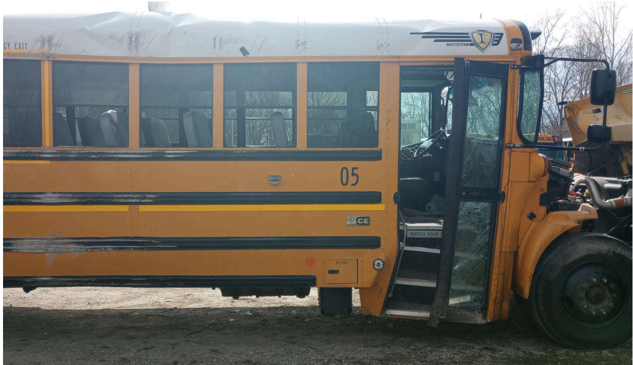
Figure 2. Damage to the right side and right-side roof of the bus. (Source: WVSP)
