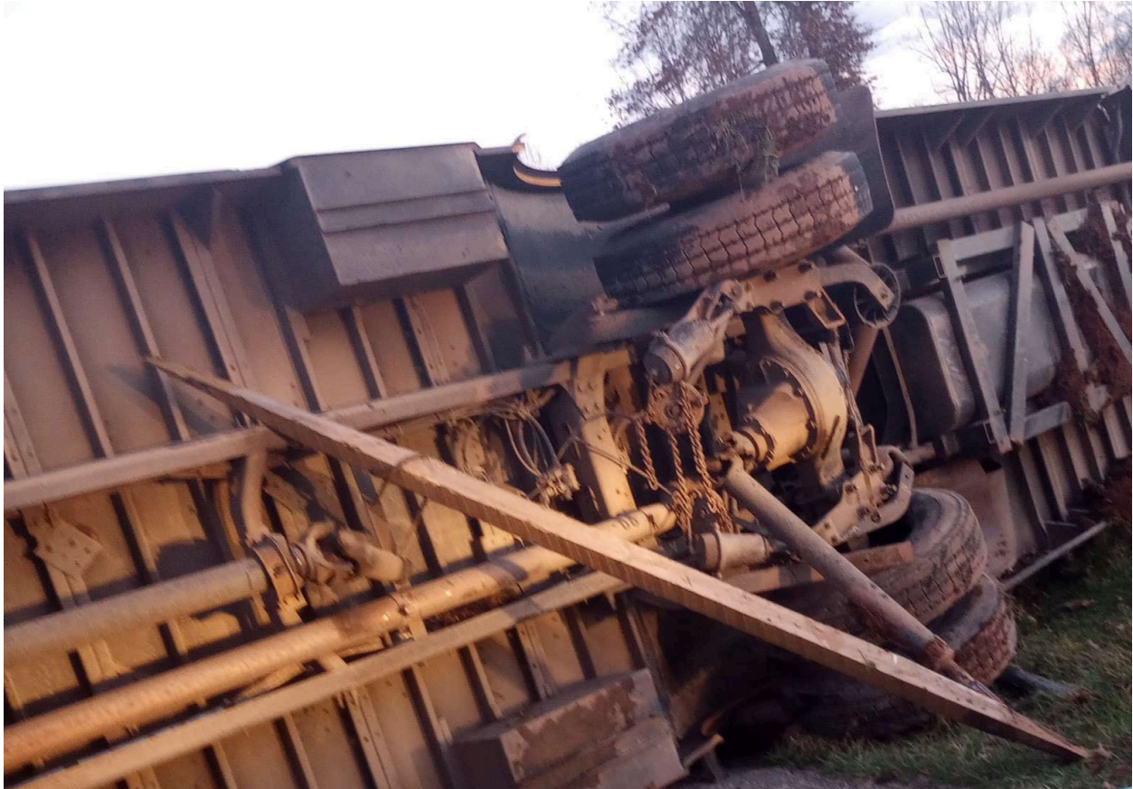
Figure 3. Undercarriage of the bus showing a fractured driveline and broken rear axle shackles (Source: WVSP)
