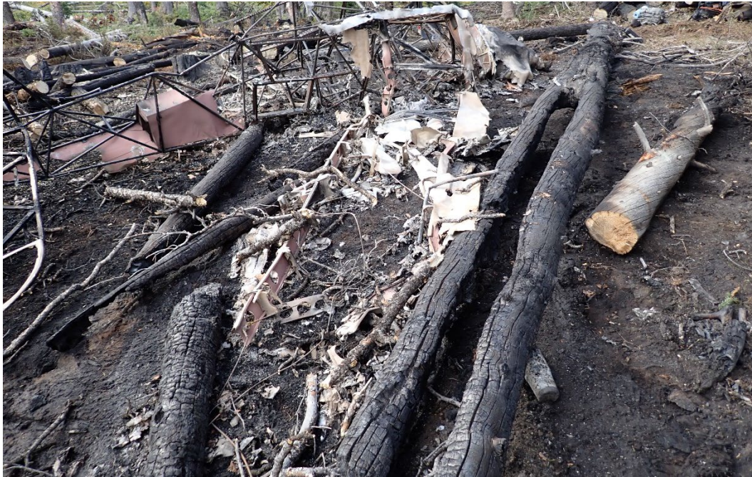
Figure 4: View of right wing thermal damage.
