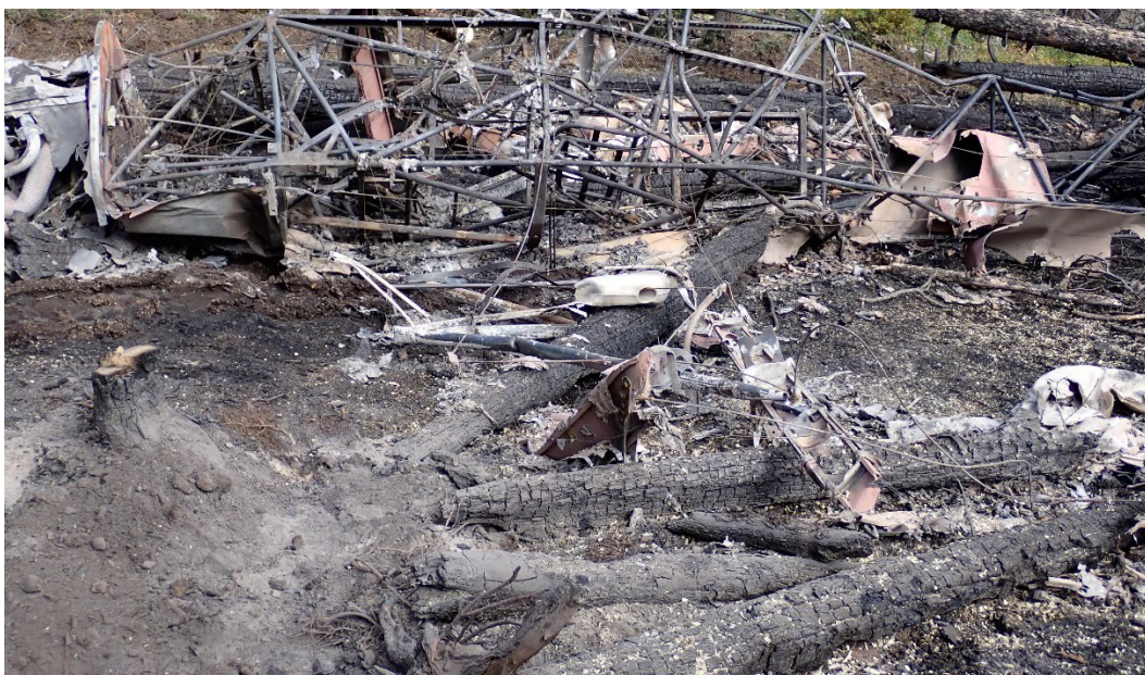
Figure 3: View of left wing thermal damage.
