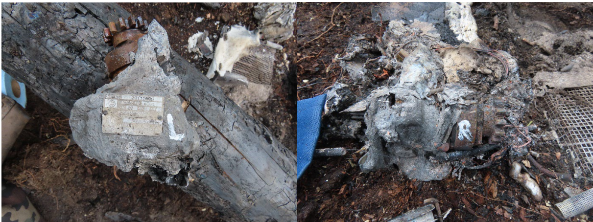
Figure 7: View of left and right magnetos.
