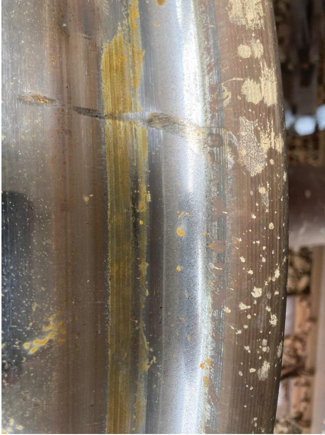
Figure 3- Exemplar photograph of broken rail Witness mark on wheel of car SHQX 10687
