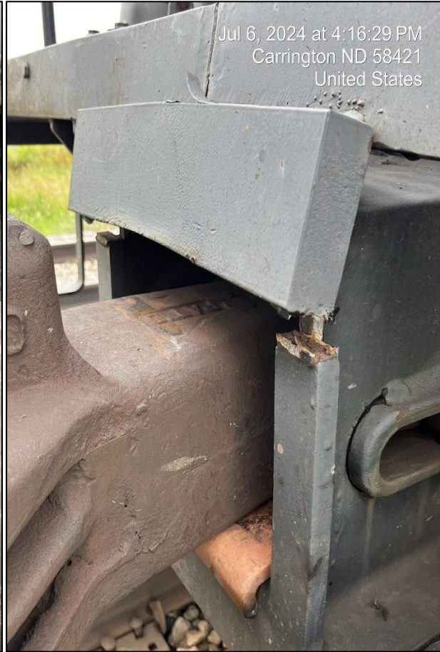
Figure 2- Exemplar photograph of a damaged buffer casting on car PROX43474
