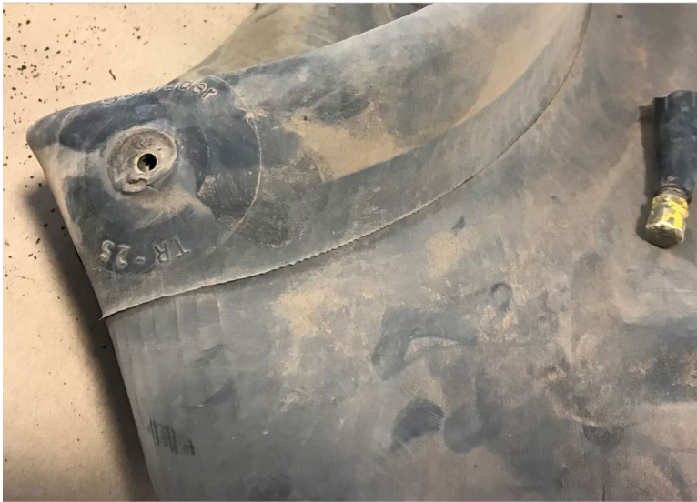
Figure 2. Sheared valve stem of the left main tire inner tube (Source: Grand Canyon Air).
