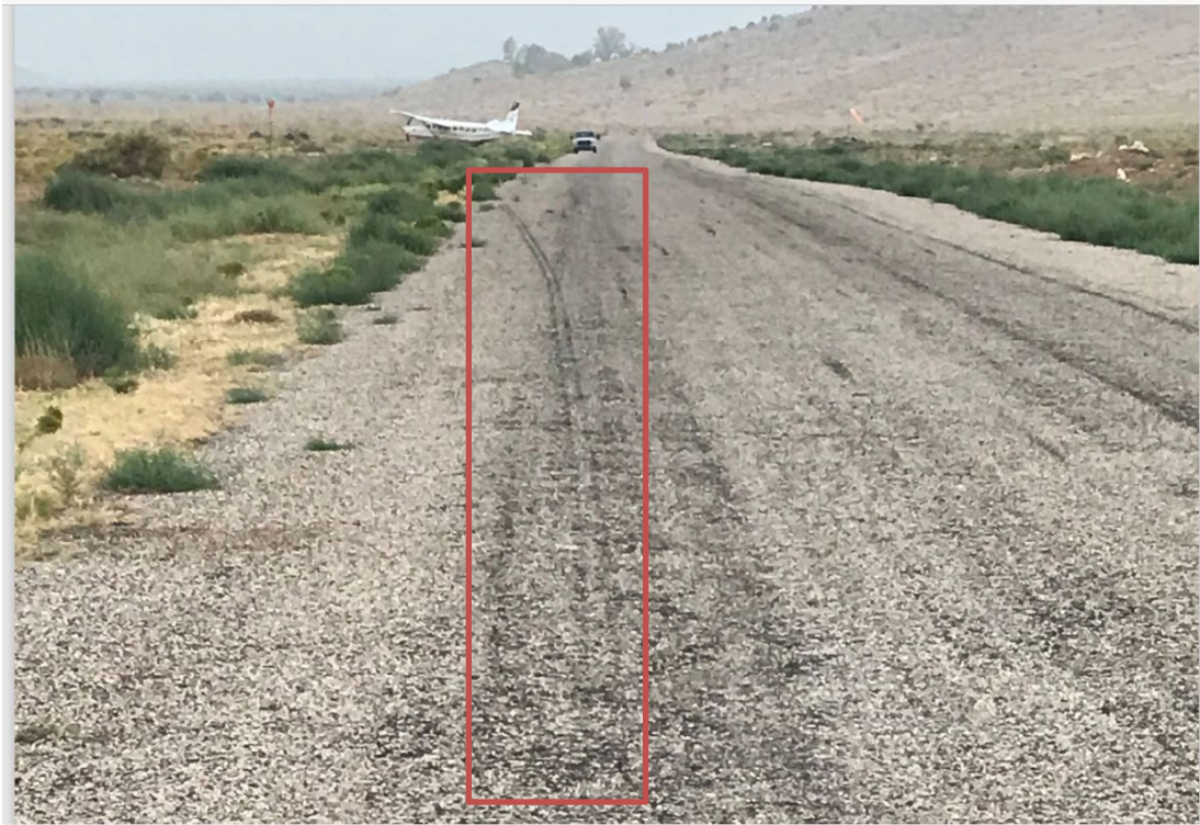
Figure 1. Tire markings on the runway with the airplane in the foreground (Source: Grand Canyon Air).
