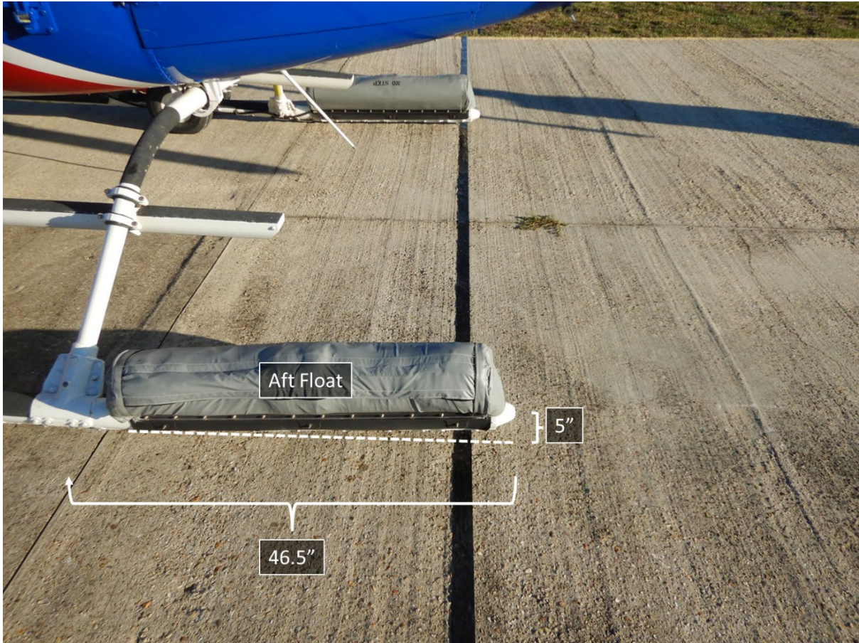
Figure 1. Exemplar helicopter showing the aft float and the aft skid section
