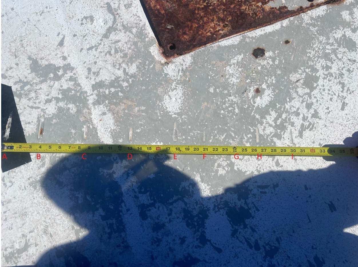
Figure 9. Photo showing the row of 9 irregularly spaced but inline gouges in the paint inside the aiming circle.
