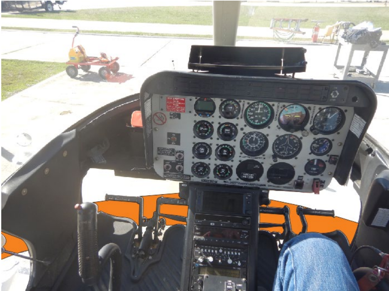
Figure 14. Photo captured with the camera positioned near the installed Appareo video recorder. The helicopter is positioned in the center of a 10 ft diameter aiming circle. The aiming circle is highlighted in orange to emphasize its location in the image only.
