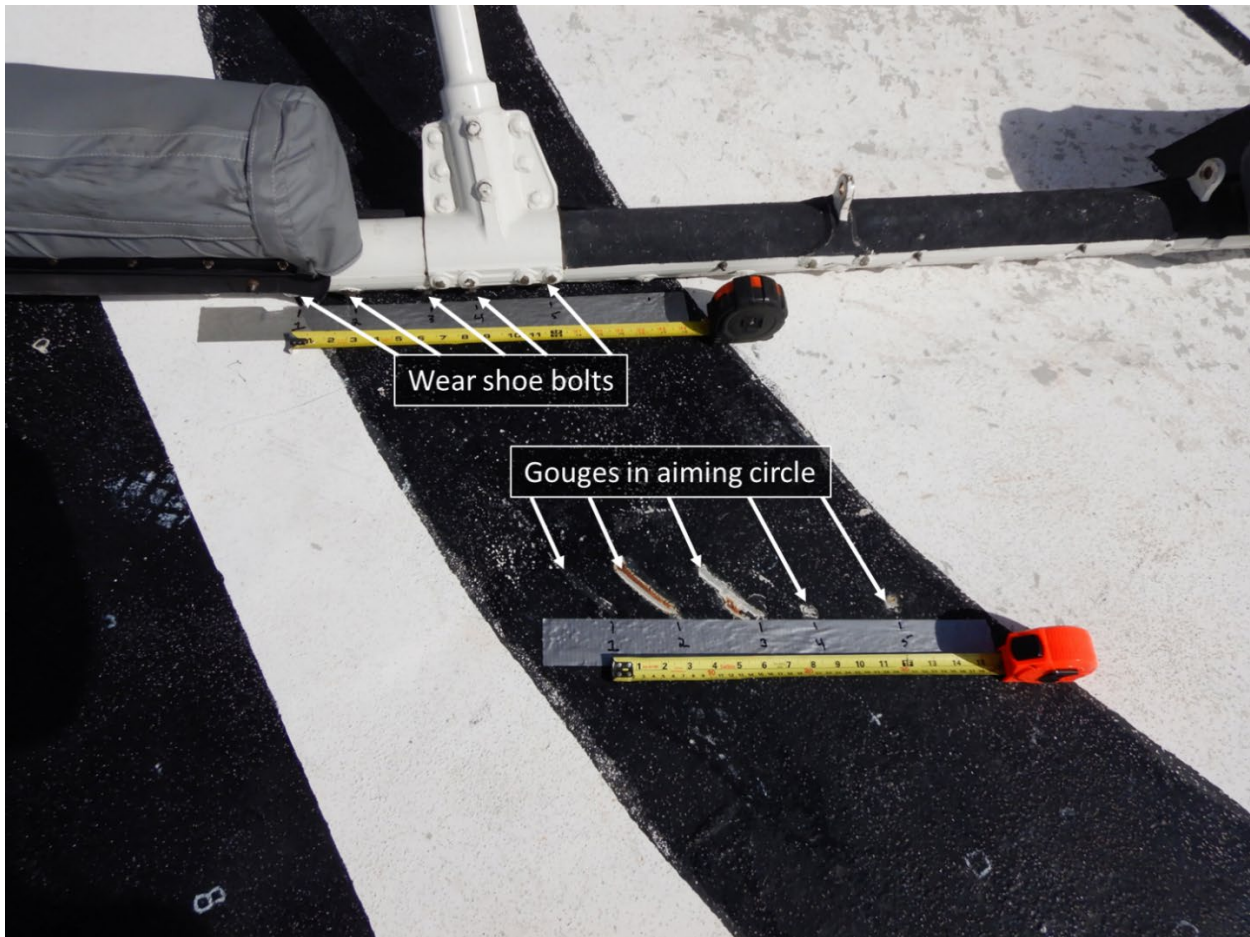
Figure 19. Image of an exemplar right skid showing the five wear shoe mounting bolts that matched the spacing of the group of five irregularly spaced gouges in the paint.
