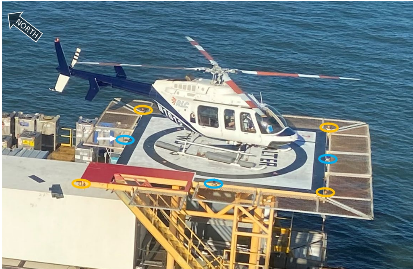
Figure 7. Close up image of an exemplar Bell 407 helicopter on the WD-106 helideck. Helideck perimeter amber lights are circled in amber, and perimeter blue lights are circled in blue. The arrow points to the light significant to the accident.
