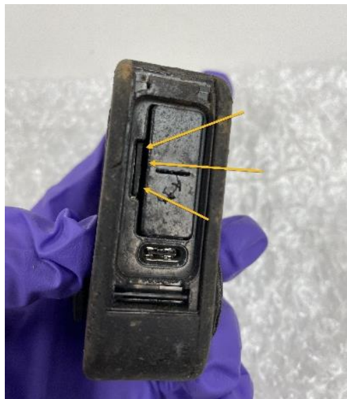
Figure 7. Memory card seated in the GoPro MAX.
