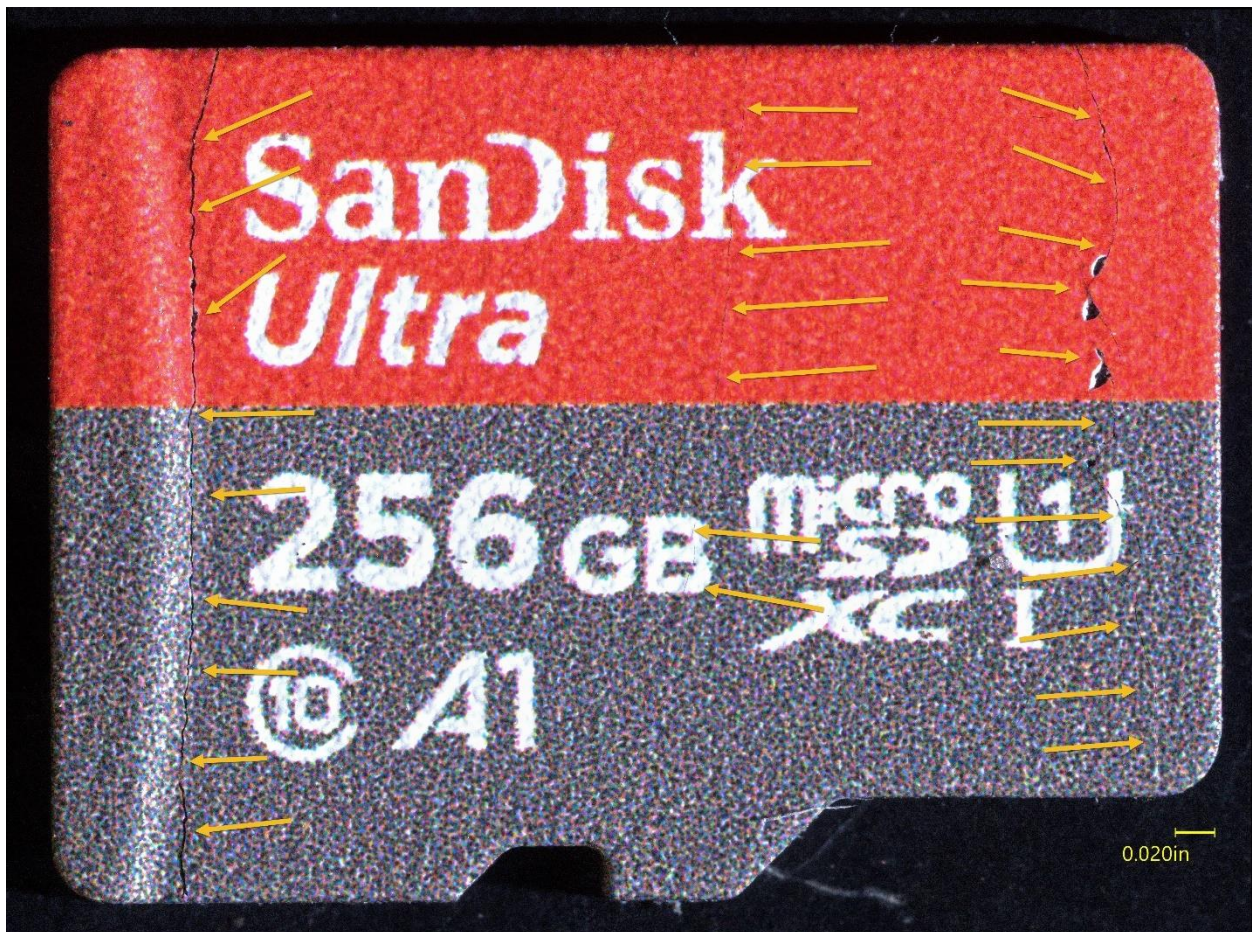
Figure 3. Annotated image showing the cracked areas of the device's associated microSD card.
