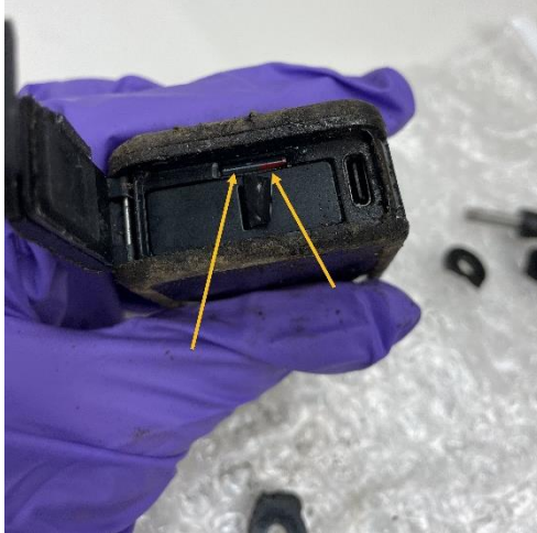
Figure 2. The microSD memory device seated in the camera's memory card chassis. The yellow arrows show the location of the seated microSD card.
