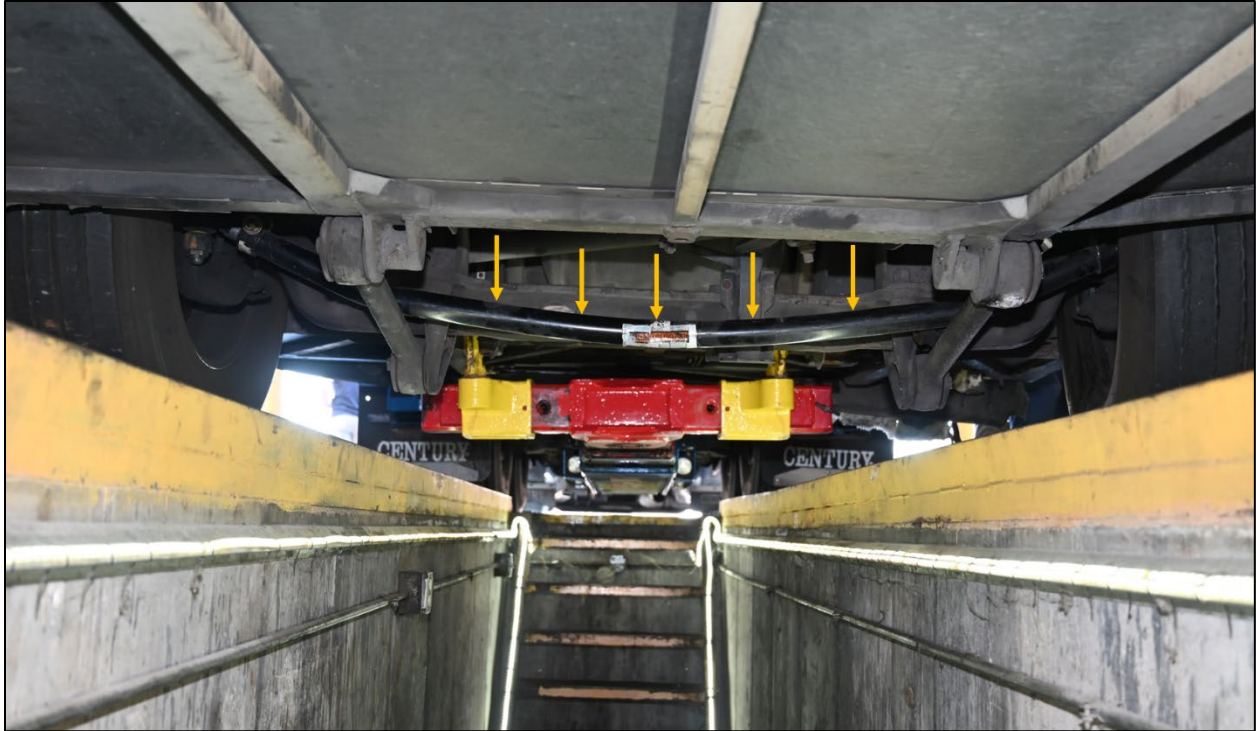
Figure 14: Motorcoach - Deformed Tie Rod
