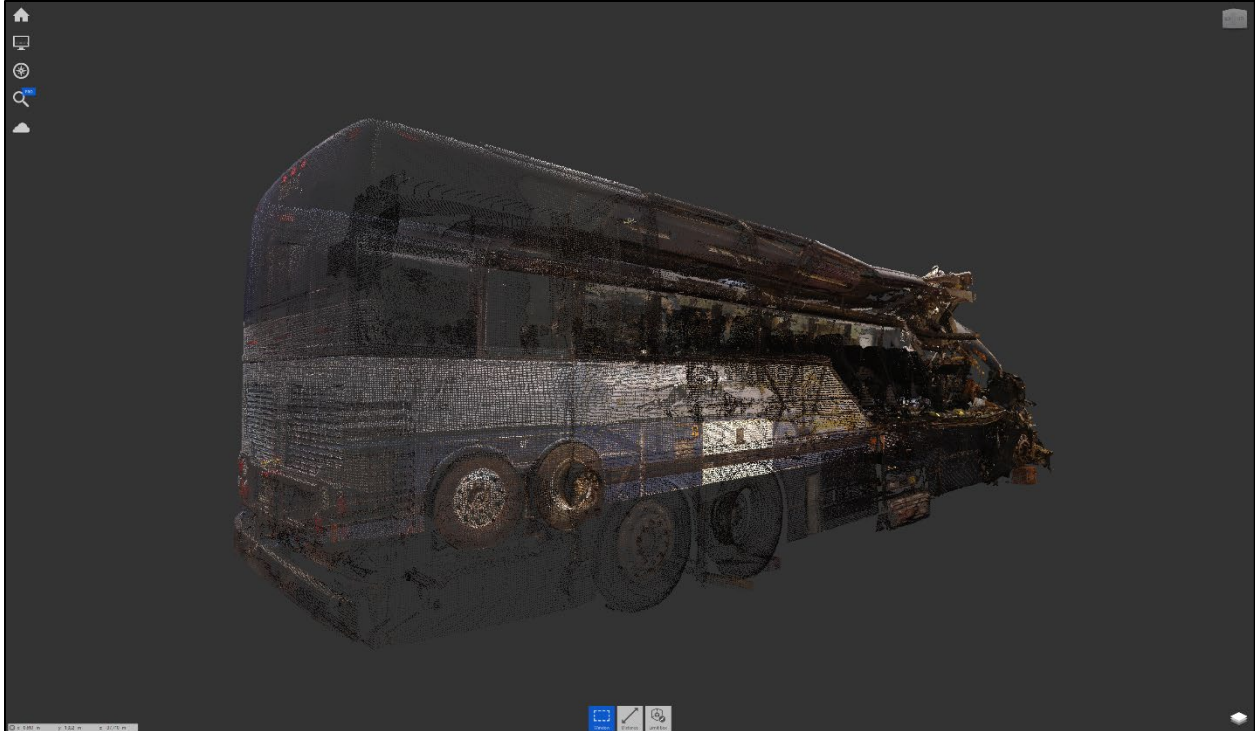
Figure 7: Motorcoach - Subject Point Cloud - Rear-Right
