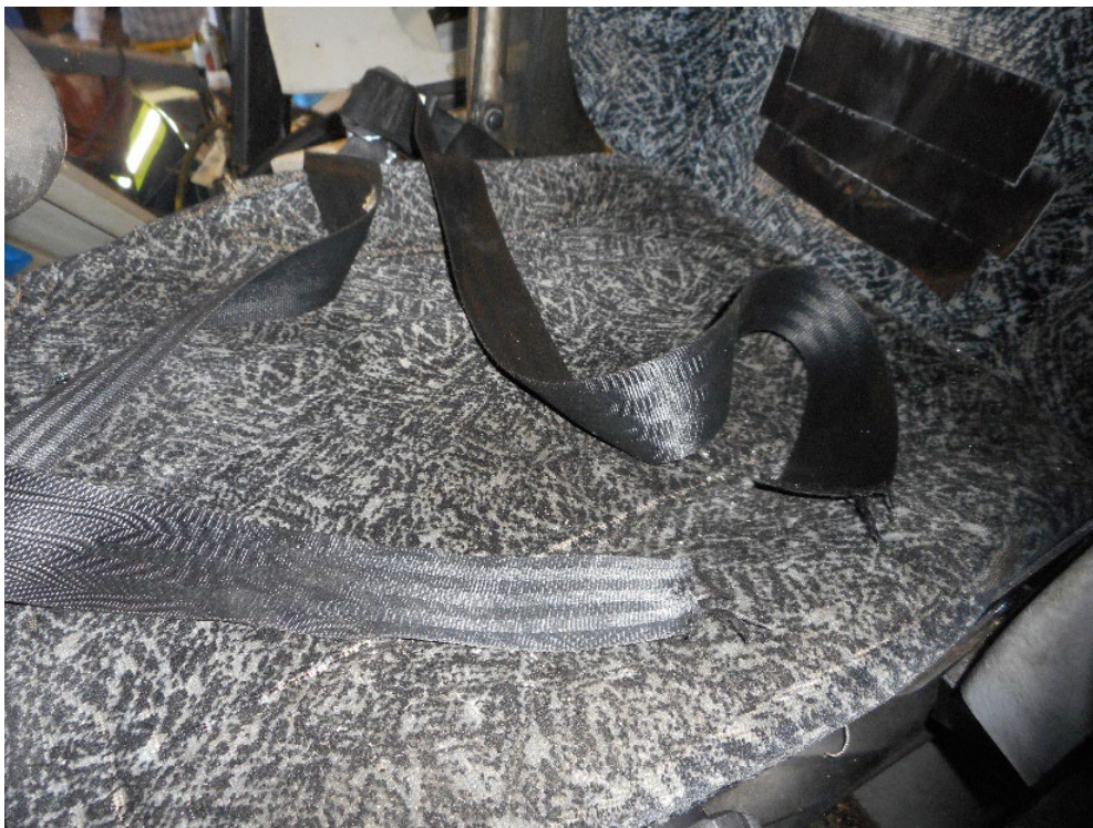
Figure 6. View of motorcoach driver's seat belt latchplate still buckled with webbing cut.
