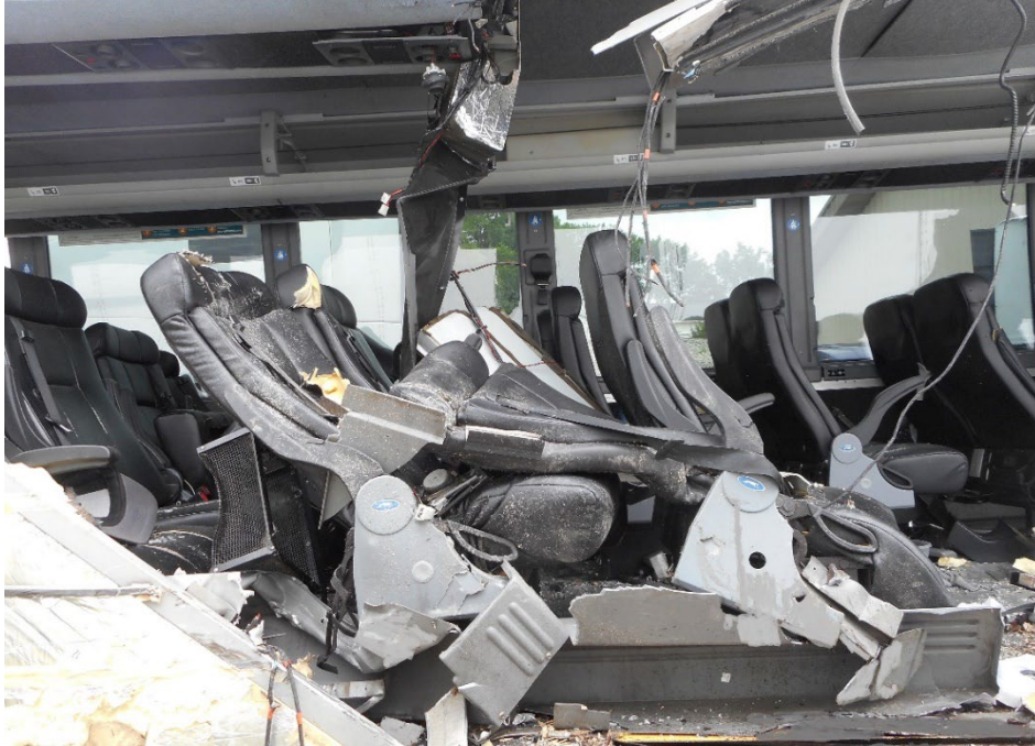
Figure 5. View of deformed seats at Rows 7-8 on right side.
