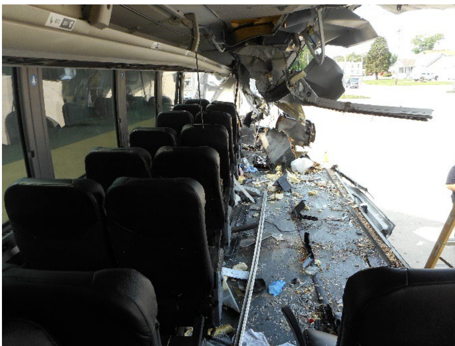
Figure 4. View of interior deformation and six missing seat rows on right side.
