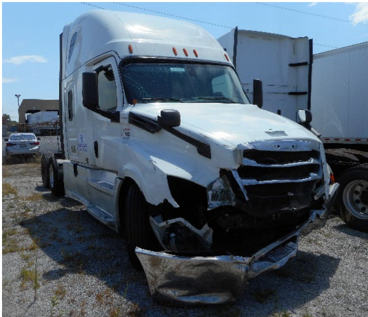
Figure 9. Frontal view of damage to Freightliner.
