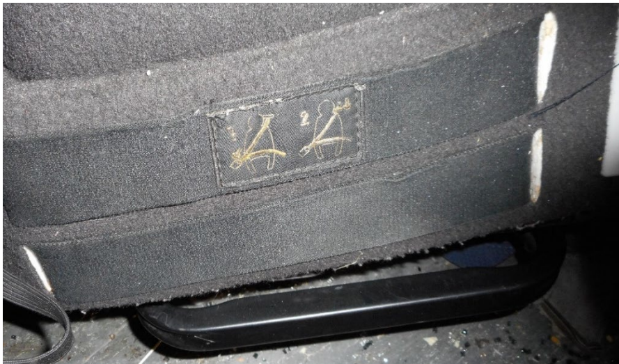
Figure 7. View of stitched in seat belt reminder to base of seatback.
