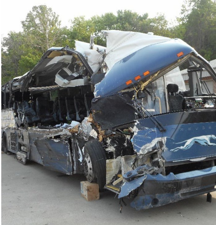
Figure 2. Front angle view of damage to motorcoach.
