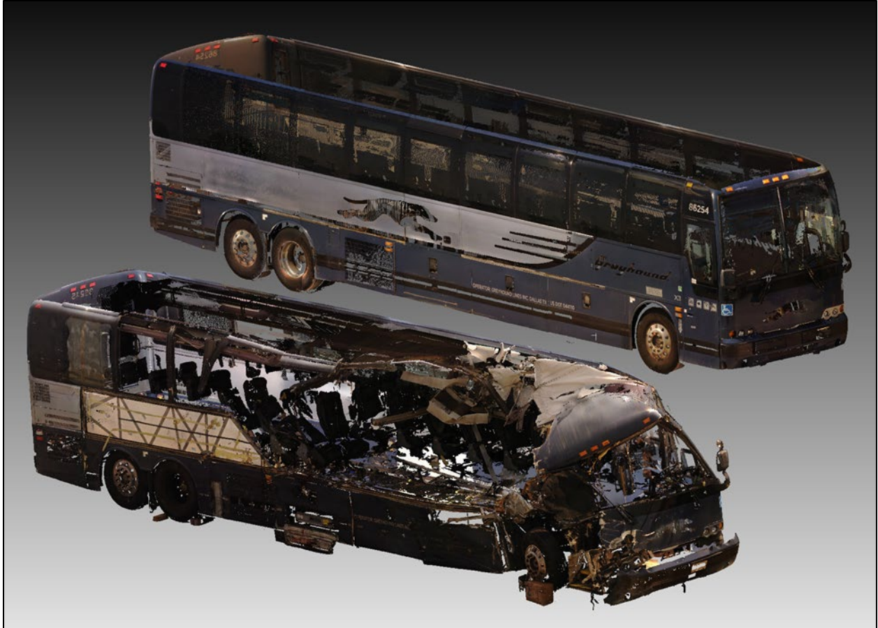
Figure 7: Three-dimensional point cloud images of the involved motorcoach and an exemplar vehicle.
