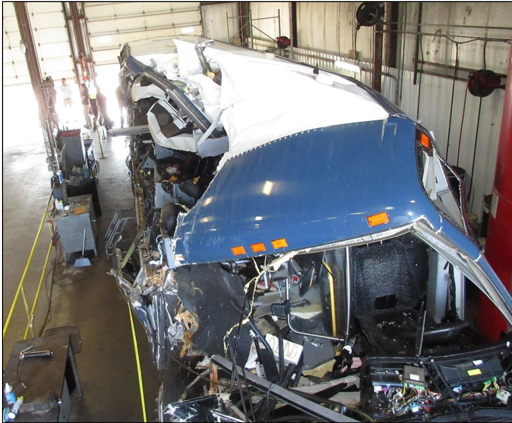
Figure 6: Photograph depicting damage to motorcoach roof.
