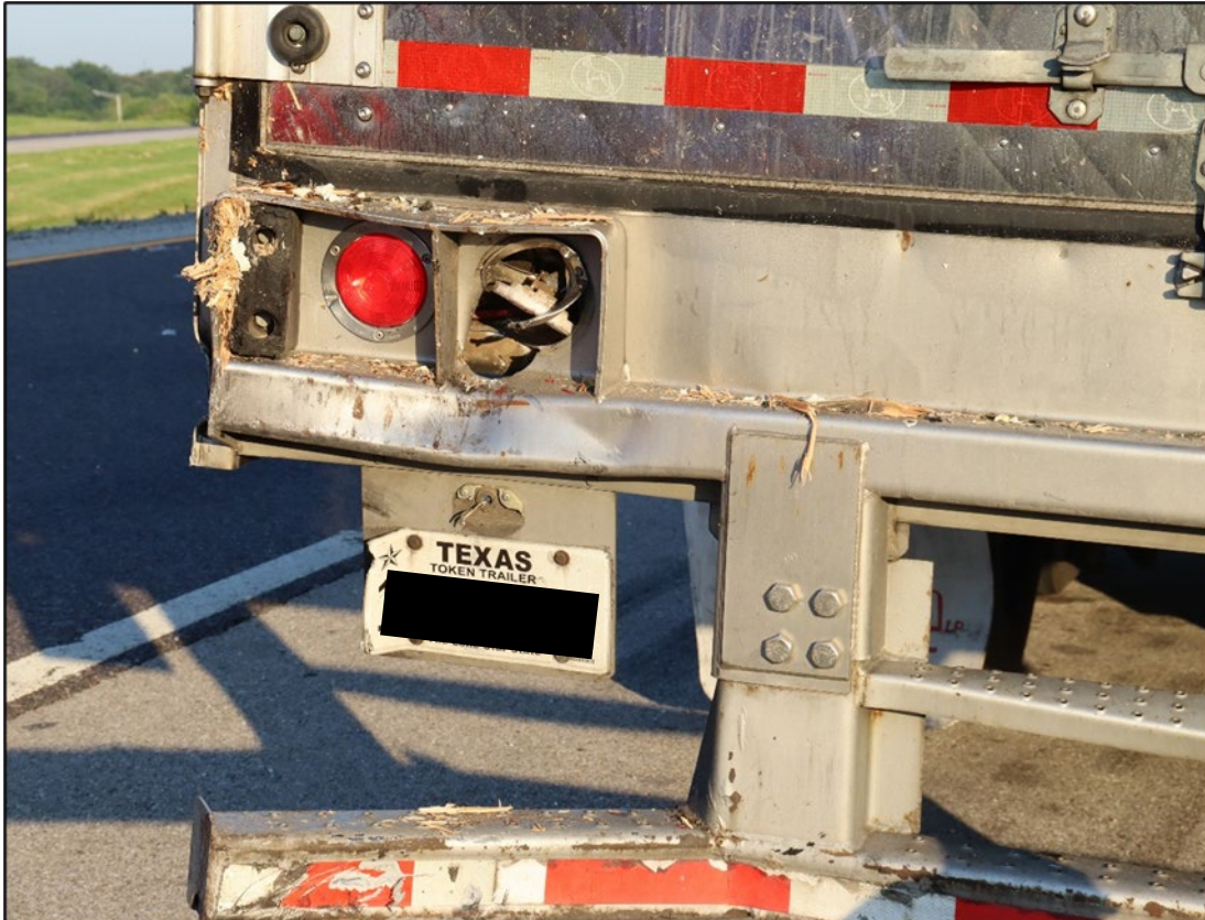
Figure 12: Photograph depicting impact damage to the driver side rear of the Great Dane semitrailer (Mack combination courtesy of ISP).
