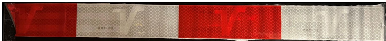
Figure 9: Photograph of retroreflective sheeting sample from rear of Vanguard semitrailer.
