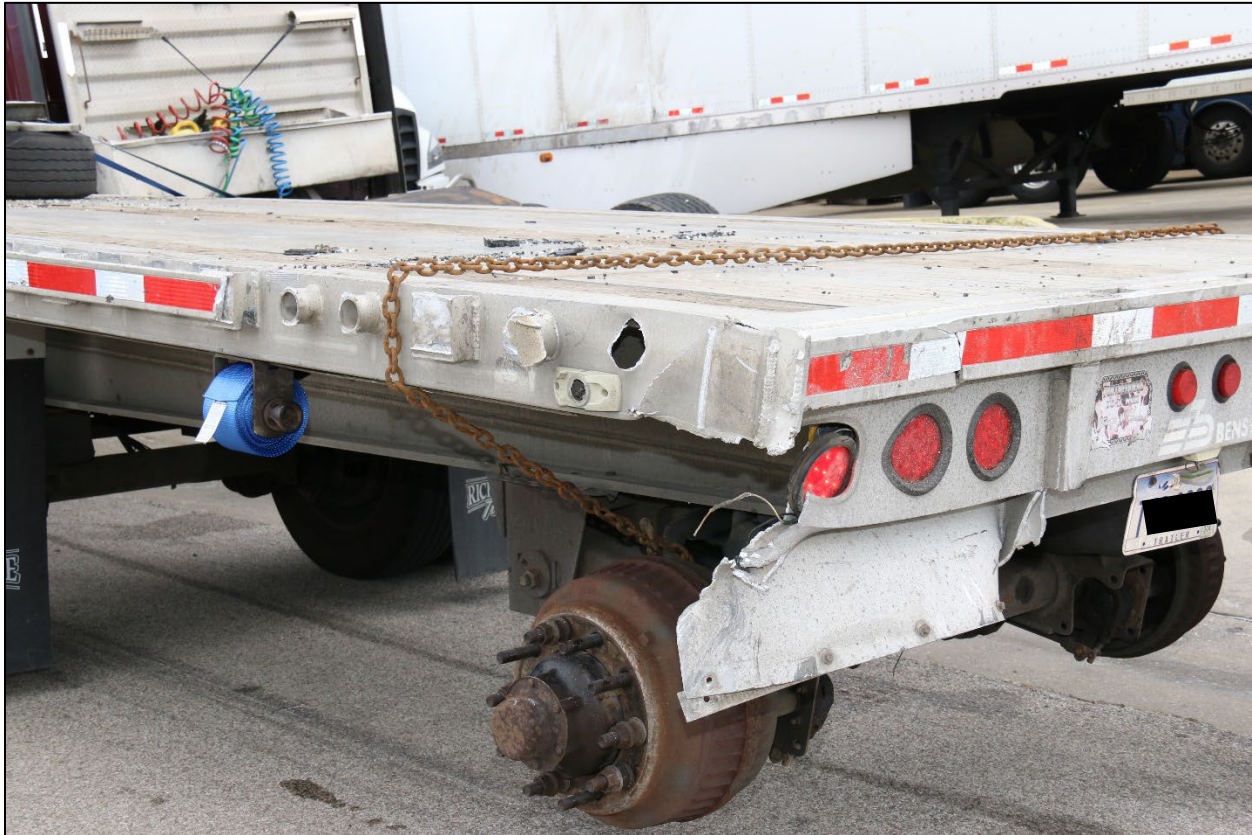
Figure 11: Photograph depicting area of first contact at the driver side rear of the Benson semitrailer (Kenworth combination).
