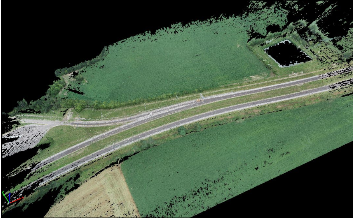
Figure 4. Generated point cloud of the crash location.
