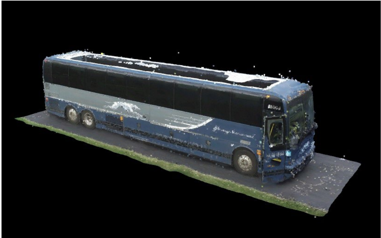
Figure 7. Generated point cloud of exemplar bus.
