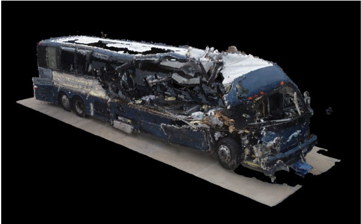
Figure 6. Generated point cloud of the involved Greyhound bus.
