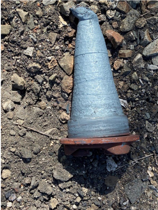
Figure 1 - Car CRDX 3017 - L1 Journal bearing.
