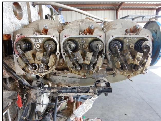
Figure 4-Right cylinders, view of overhead components.
