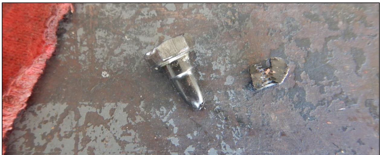
Figure 8-Portions of the connecting rod bolt and nut.
