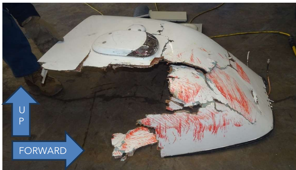
Figure 2. The forward upper cowling exhibiting red paint transfer.
