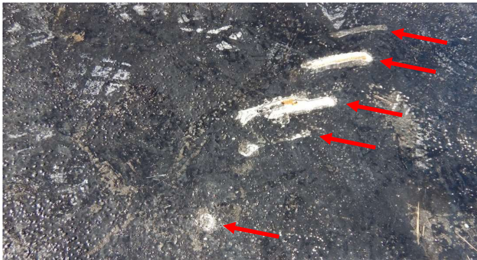
Figure 4. A group of impact marks on the helipad with an arc-like appearance.
