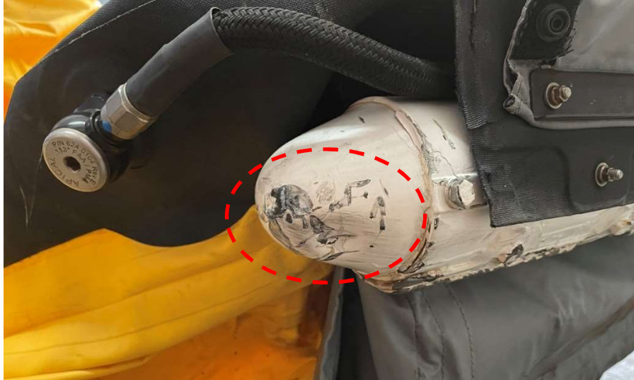
Figure 3. Damage to the conical end cap on the aft end of the right landing skid.
