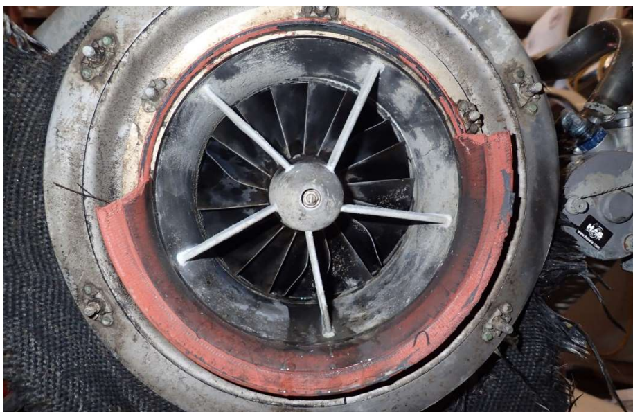
Figure 13. The compressor impeller blades viewed through the engine inlet. (Image courtesy of Rolls-Royce)
