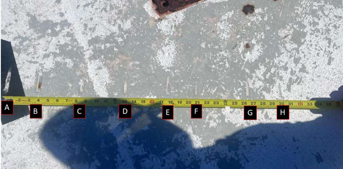
Figure 5. A group of impact marks on the helipad with a linear appearance.
