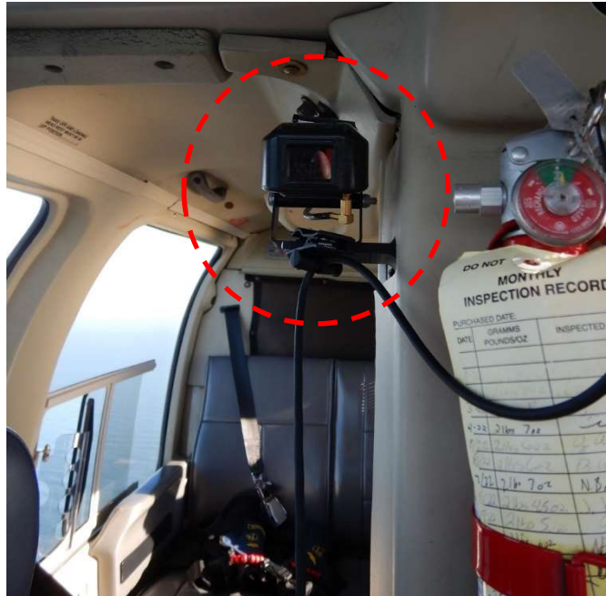
Figure 14. An Appareo Vision 1000 installation on an exemplar Bell 407. The viewpoint of this image is forward-looking-aft.
