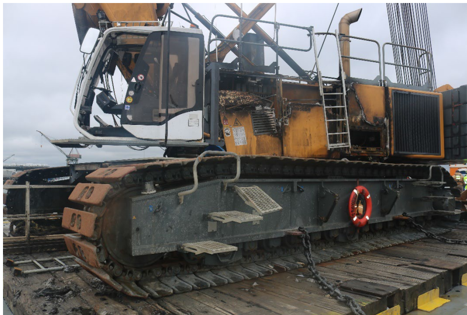
Figure 5. The damaged crane postfire. (Source: Coast Guard)
