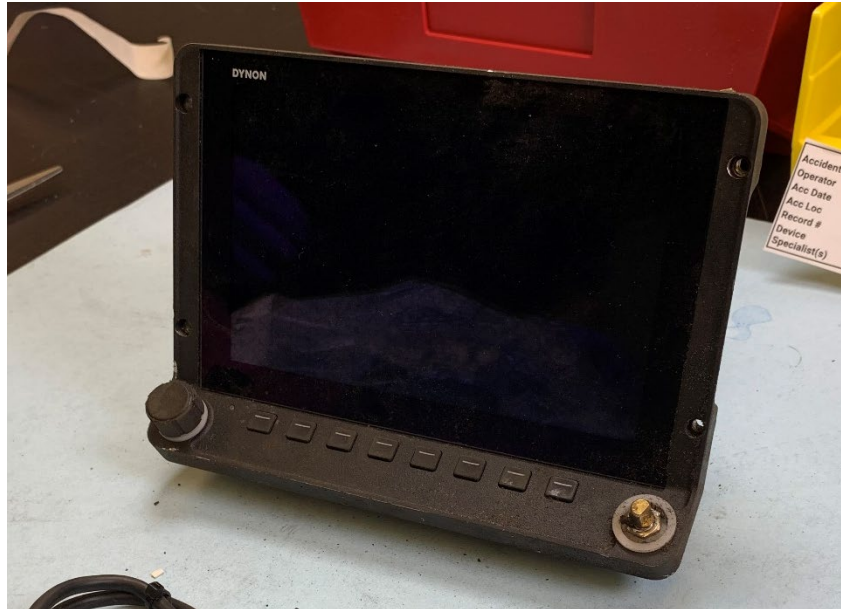
Figure 2. Dynon Skyview SV-HDX800 as received by vehicle recorder laboratory.
