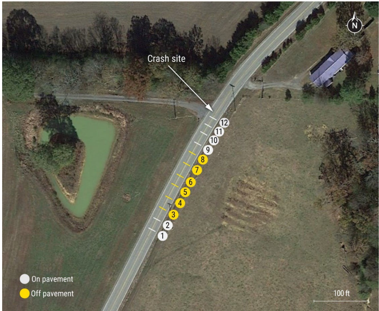
Figure 12. Aerial photo of SR-58 at the crash site, with overlaid markers. The yellow numbers indicate locations where the right-most tire mark was found in the earthen v-ditch, and the white numbers indicate that the truck's right-most tire mark was located on the pavement.
