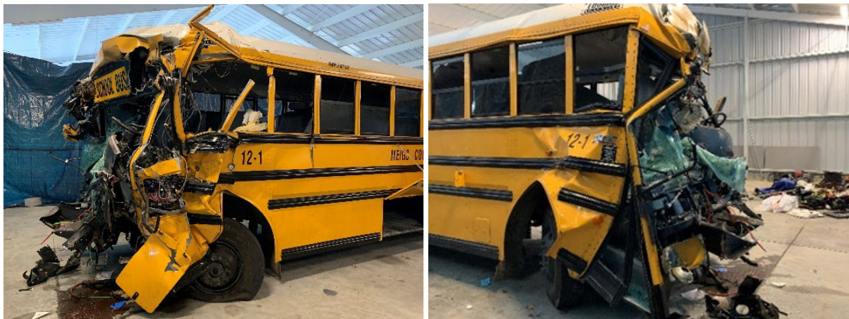
Figure 9. Crash damage to the driver side and right side of the school bus.
