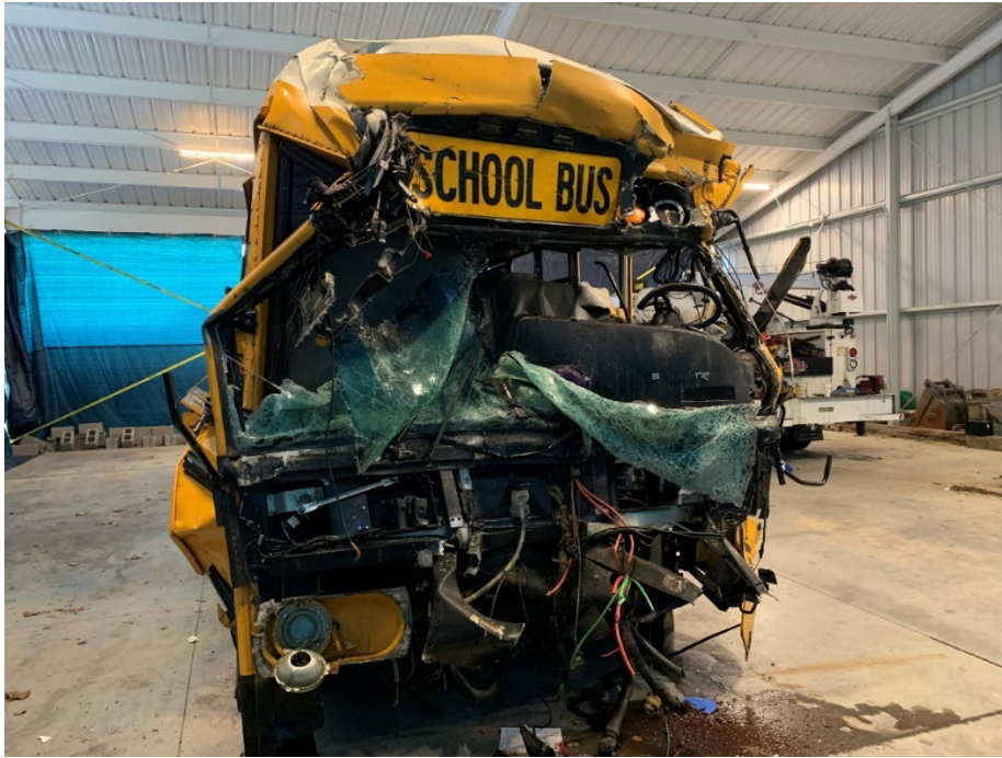
Figure 8. School bus front damage.
