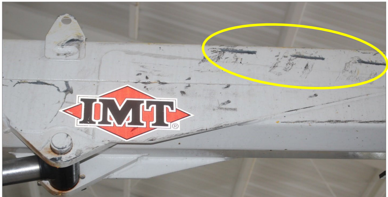
Figure 7. Damaged crane arm of service truck.
