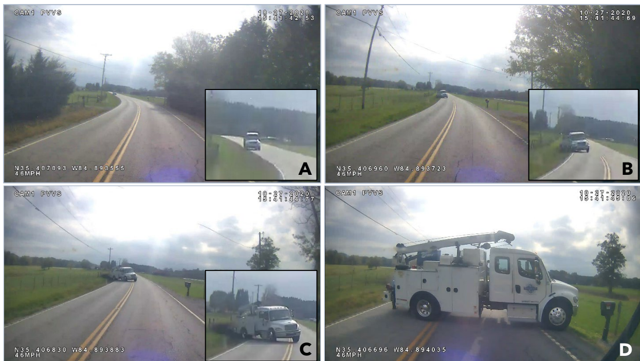
Figure 3. Video frames, captured by the outward-facing camera onboard the school bus, showing the truck departing the road (A), returning to the road (B), and crossing into the travel lane of the bus (C & D). The inserts are close-up images of the truck.
