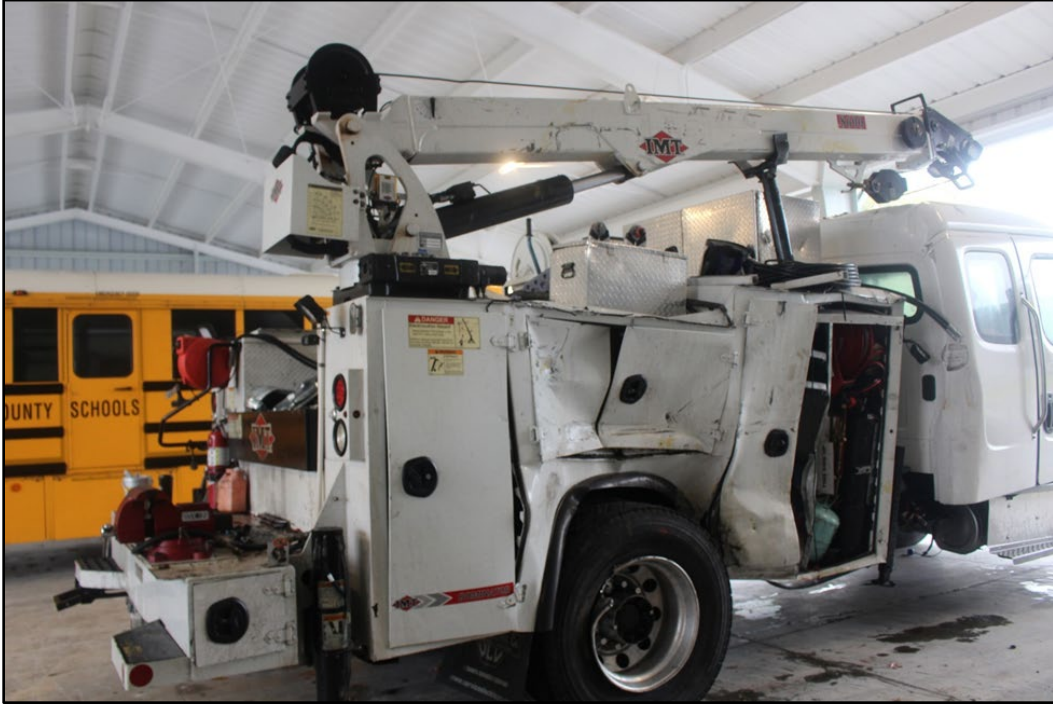
Figure 2. Damage to right side of truck. (Source: Tennessee Highway Patrol)
