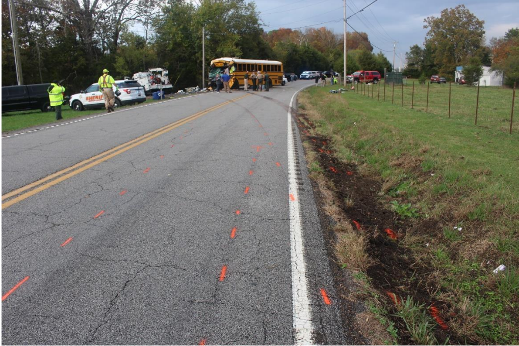
Highway Factors Photo 5 – Another view of SR-58 looking to the north standing in the northbound lane with the accident school bus located in the background. The orange dash lines denote the approximate location of the tire marks of the service truck (Source: THP)
