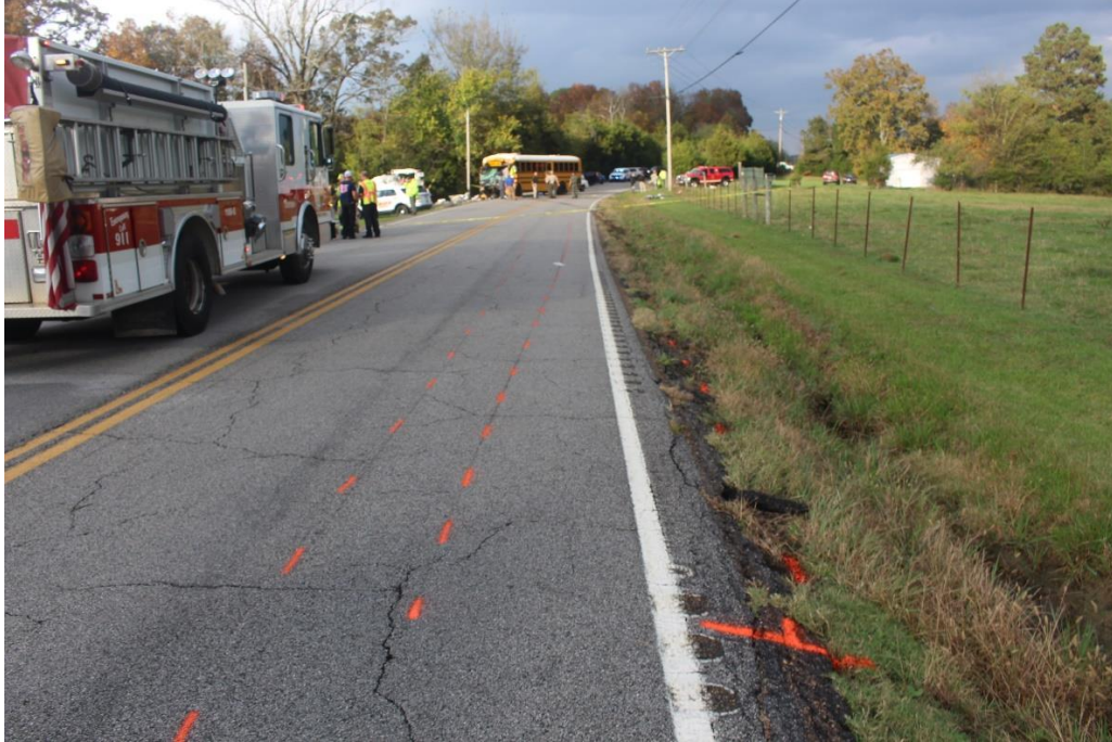
Highway Factors Photo 3 – View of SR-58 looking to the north standing in the northbound lane with the accident school bus located in the background. The orange dash lines denote the approximate location of the tire marks of the service truck (Source: THP)
