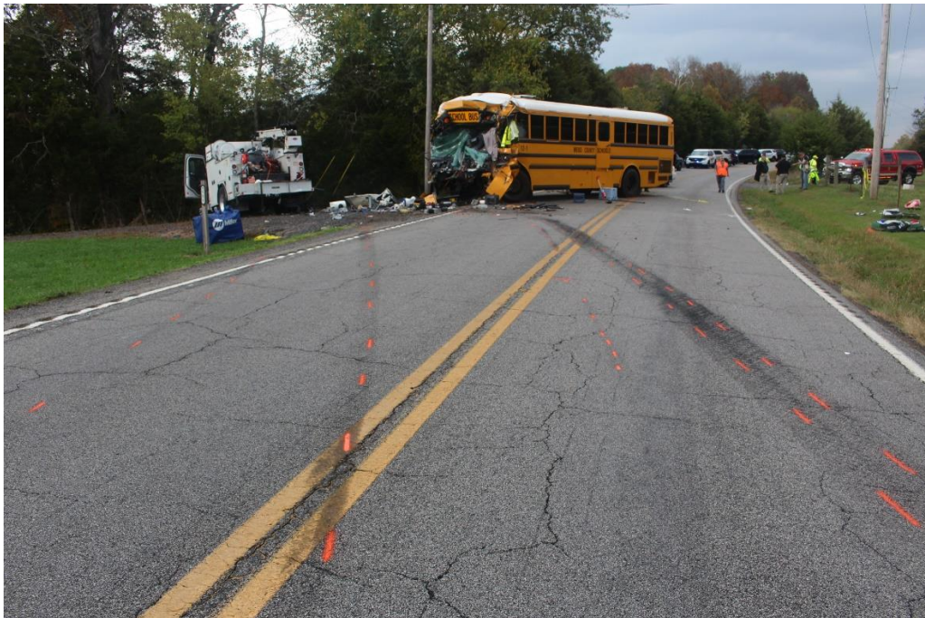
Highway Factors Photo 6 – Another view of SR-58 looking to the north standing in the northbound lane with the accident school bus and service truck located in the background. The orange dash lines denote the approximate location of the tire marks of the service truck (Source: THP)
