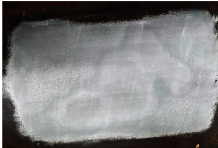
Figure 4.0 - Acid Etched Hard Spot
